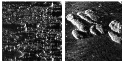
Figure 1.5. Examples of types of sea bottom with rocks from a side-looking sonar image. Left. A cluttered area with small rocks. Right. Big rocks.
