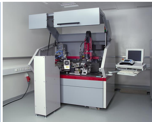
Fig. 3. (a). Graphic illustration of the micro-factory concept; and (b). The manufacturing platform used for testing the concept (POLYTUBES consortium and Sysmelec of Switzerland)
