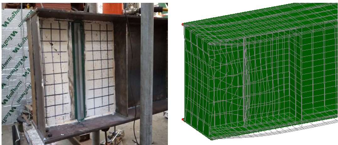
Figure 5.42 Test and FEA modes of failure of GFRP-strengthened specimen B2
