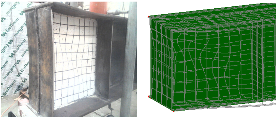
Figure 5.41 Test and FEA modes of failure of un-strengthened specimen B1
