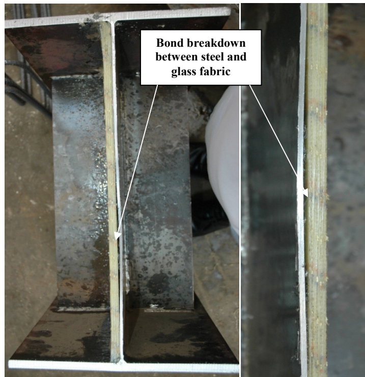
Figure 3.56 Bond breakdown between steel and glass fabric in specimen B4
