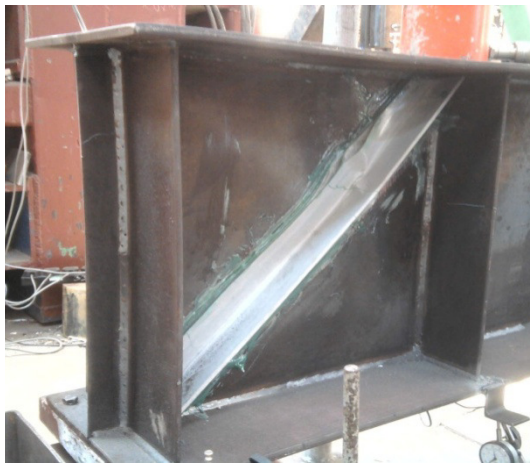
Figure 5.44 Test and FEA modes of failure of GFRP-strengthened specimen B6
