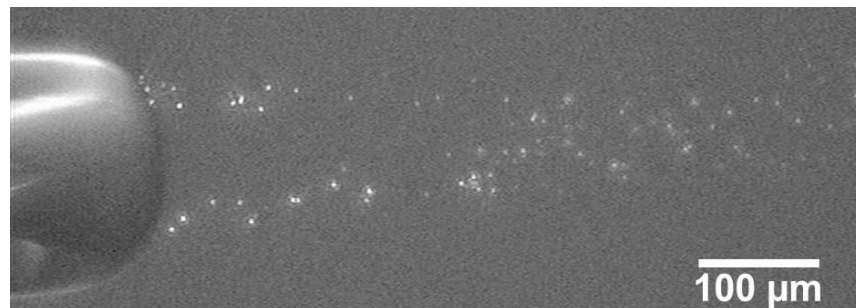
Figure 4.14. Side profile of the lensed MCF showing 1047 nm light scattered from 1.3 \mu\text{m} polystyrene microspheres in water.
