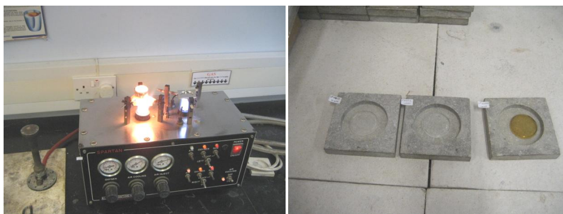
Figure 3.1: Fused bead preparation and prepared fused bead ready for XRF
