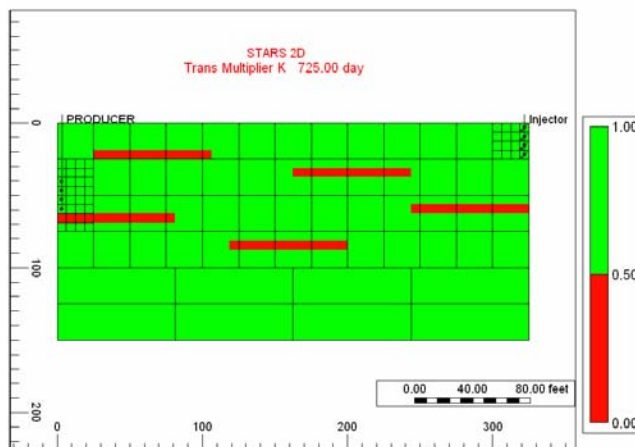
Figure 6.32: Location of discontinuous impermeable shale layers in the vertical well configuration with aquifer support
