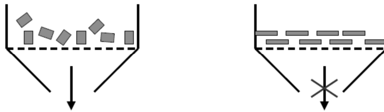
Figure 2.1.17 - Cubes allow for free flowing filtrate, plates can slow or even block filtration [29]
