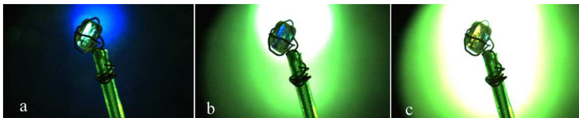
Figure 3.9 - Determination of seed handedness a) initially crossed polarizers b) second polarizer rotated clockwise c) further rotating second polarizer clockwise
