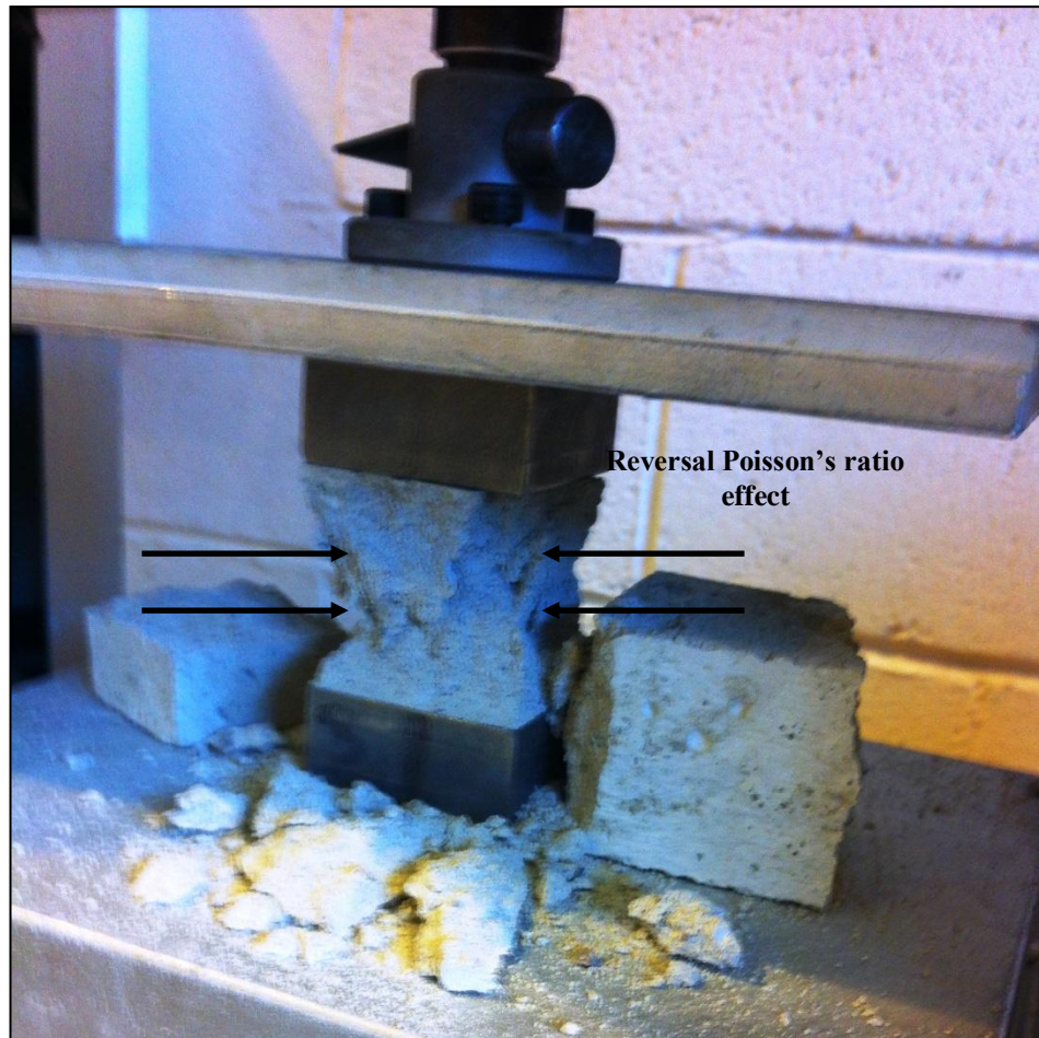
Figure 5.2: Stress caused by platen restraint on a mortar cube during testing with metal pad
