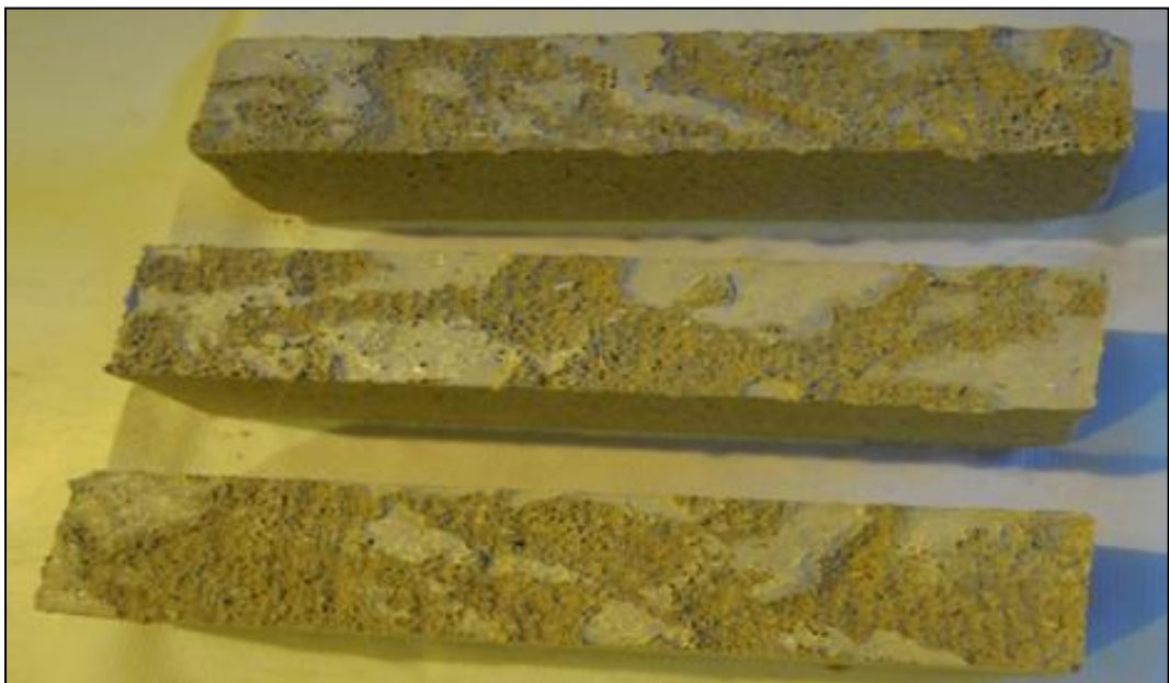
Figure 3.16: Shrinkage cracks in mortar specimens of 33°C - 90%RH
