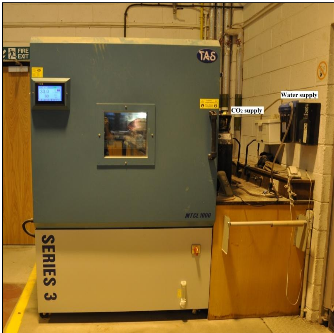
Figure 3.12: TAS Environmental Curing Cabinet
