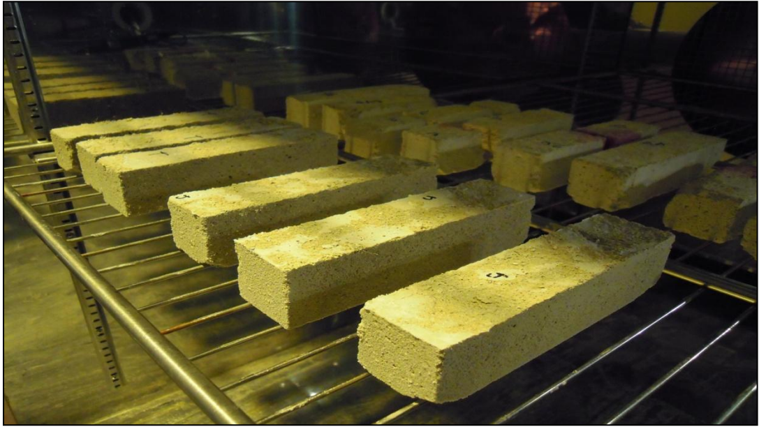
Figure 3.13: View inside of the TAS Environmental Curing Cabinet
