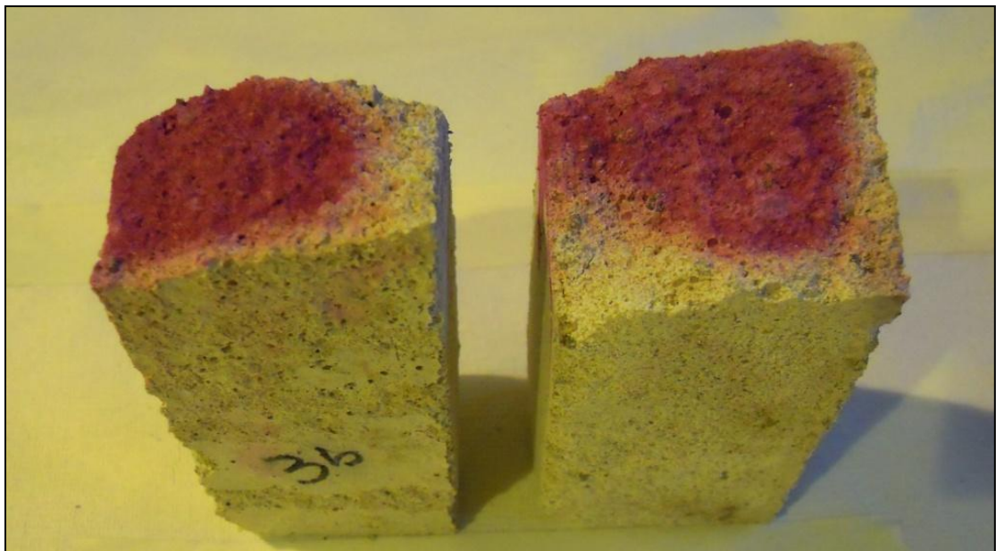
Figure 3.18: Carbonation Depth Test
