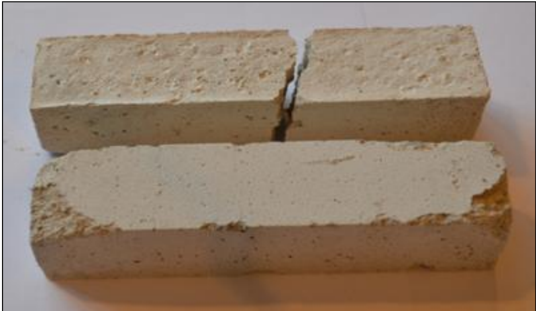
Figure 3.14: Shrinkage cracks in mortar specimens of 20°C - 60%RH
