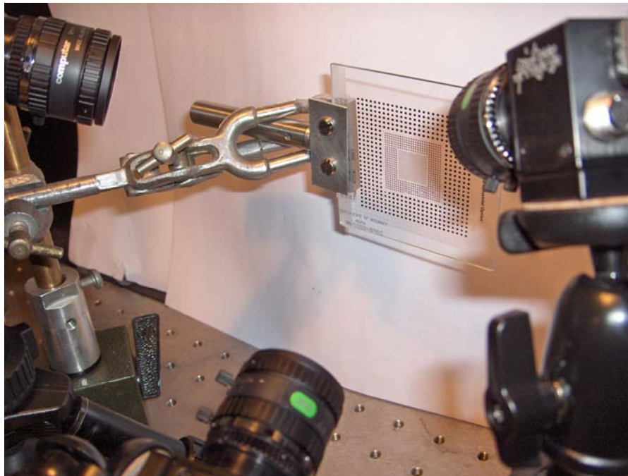
Figure 20: Experimental setup for fixed camera photogrammetry.
