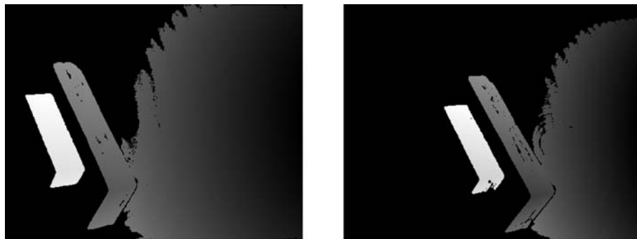
Figure 73: Phase maps of the same object from perspectives showing previously occluded surfaces.
