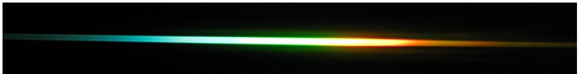
Figure 4.15: Visible wavelength component of the supercontinuum from PCF-24 dispersed through a prism.
