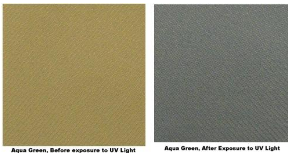
Figure 3.14 Polyester fabric dyed with Aqua Green by the exhaustion method
