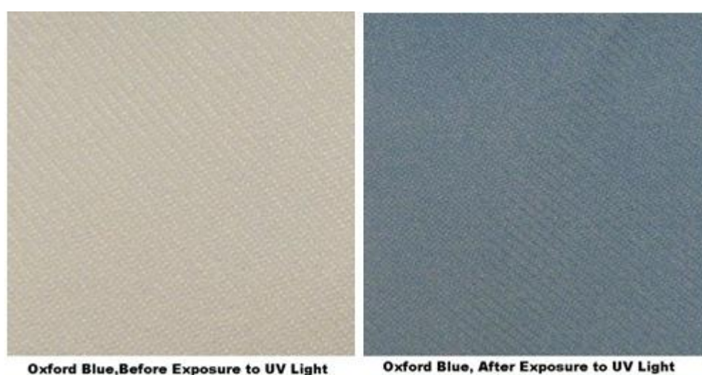
Figure 3.15 Polyester fabric dyed with Oxford Blue by the exhaustion method
