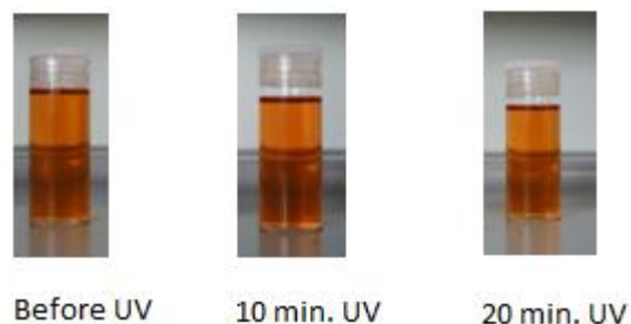
Figure 9.27 Colour development on UV exposure of a solution of azospirooxazine dye 2 in dichloromethane
