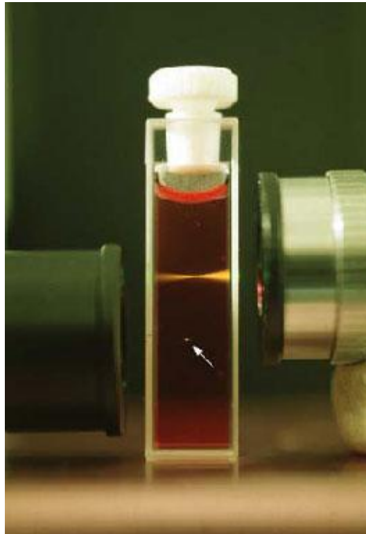
Figure 2.1. Linear absorption vs nonlinear absorption. The top beam, incident from the right shows fluorescence with a single photon absorption regime whereas the bottom beam incident from the left shows the smaller, point-like fluorescence resulting from a nonlinear 2-photon absorption process. Picture taken from B. Amos [36].
