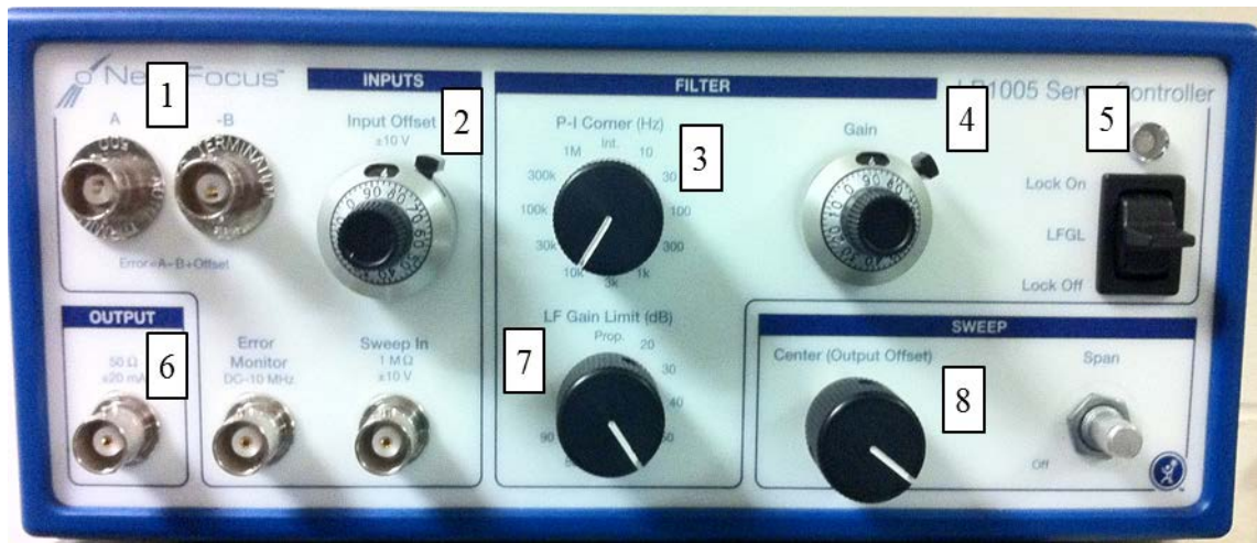
Figure 4.8. Front panel of the New Focus LB1005 PI amplifier. 1, input ports; 2, input offset control; 3, PI corner frequency control; 4, proportional gain control; 5, gain regime control; 6, output port; 7, low frequency gain control; 8, output offset control.
