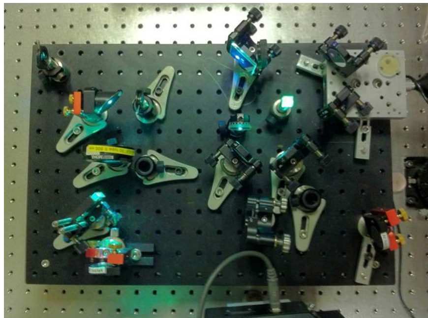
Figure 3.26. Schematic (top) and photograph (bottom) of the XFROG experiment.
