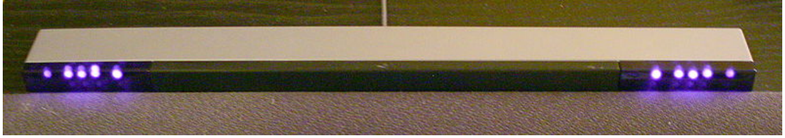
Figure 4.3 - The Wii Sensor Bar with its infrared LEDs. N.B. The LEDs are not visible to the naked eye, but most digital cameras are sensitive to infrared sources, showing them as purple light. Image from [41].
