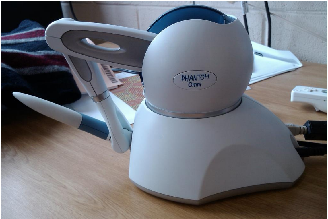
Figure 4.1 - The haptic pen used for our investigation, a Phantom Omni
