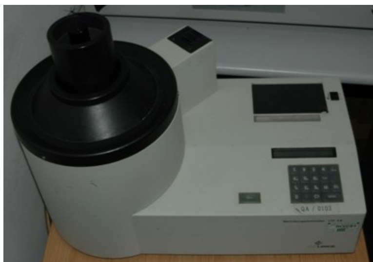
Figure 3.1.1.1 Dr. Lange LTP6B haze meter.
