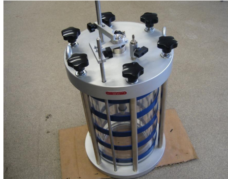
Figure 4.4: Features of the double-wall cell
