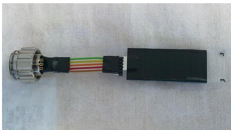
Figure 7.1 Microelectrode showing the connections to an Amplikon 10 pin connector.
