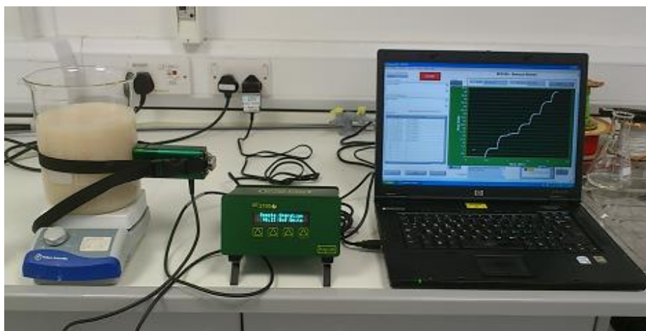
Figure 8.1 Experimental set up showing the Buglab BE2100 optical sensor.
