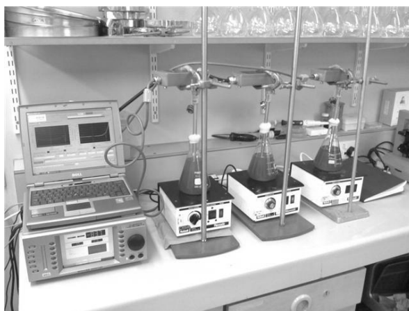
Figure 3.2 Biomass monitor model 220 from Aber Instruments using three probes at the same time.
