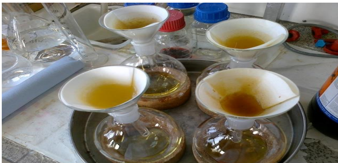
Figure 2-10 Filtering tissues using GF/C Filter paper
