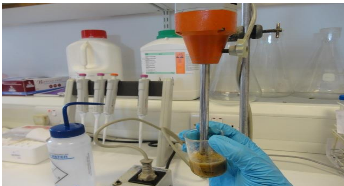
Figure 2-15 Homogenising the tissues, using a homogeniser (Ystral GmbH, Re D-7801, Dottingen, Type X 1020, 220V, 05HZ, Nr 3132, 1.25 A, 260 W, 25000 upm)
