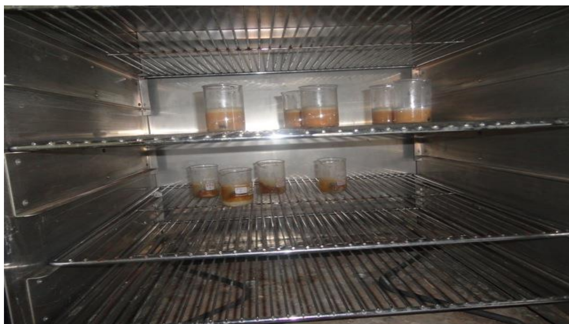
Figure 2-16 Drying the tissues in an oven at 50°C
