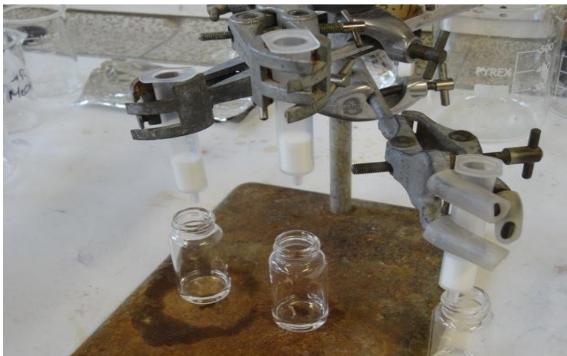
Figure 2-13 Fractionating PW sample using Strata C18-E to remove non-polar compounds
