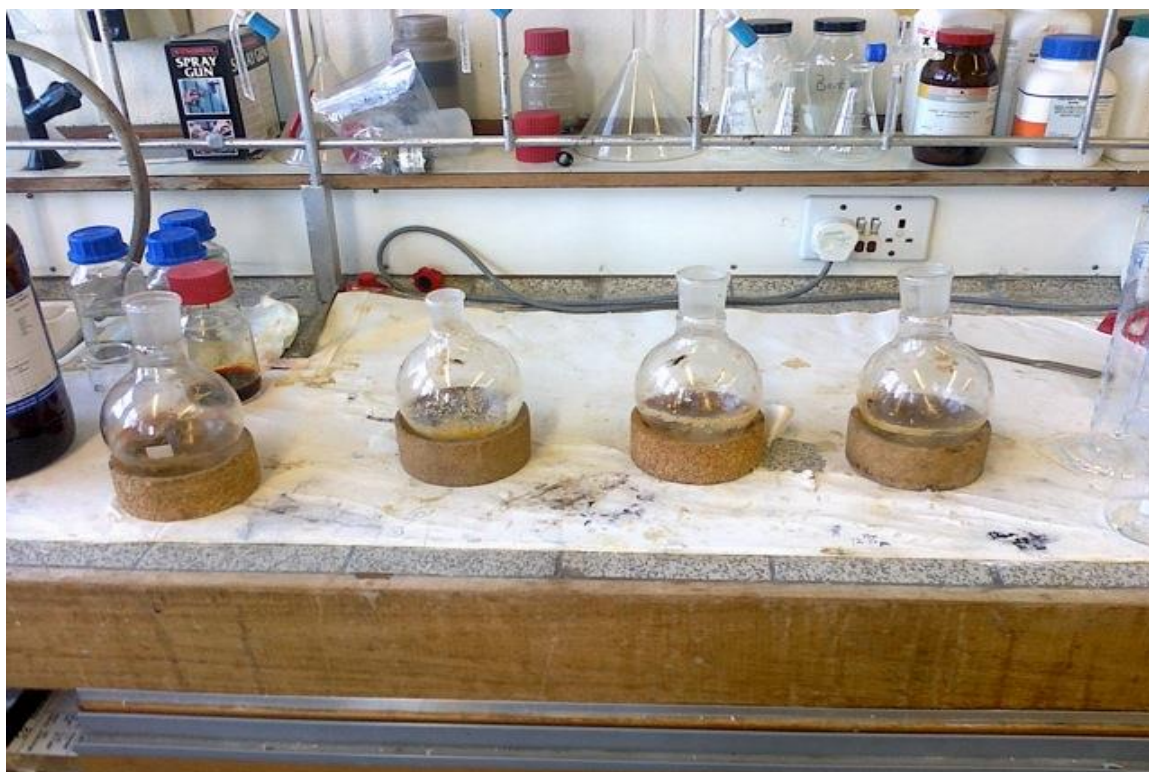
Figure 2-9 Round bottomed flasks after refluxing the tissues for 4 hours and preparing for filtration.
