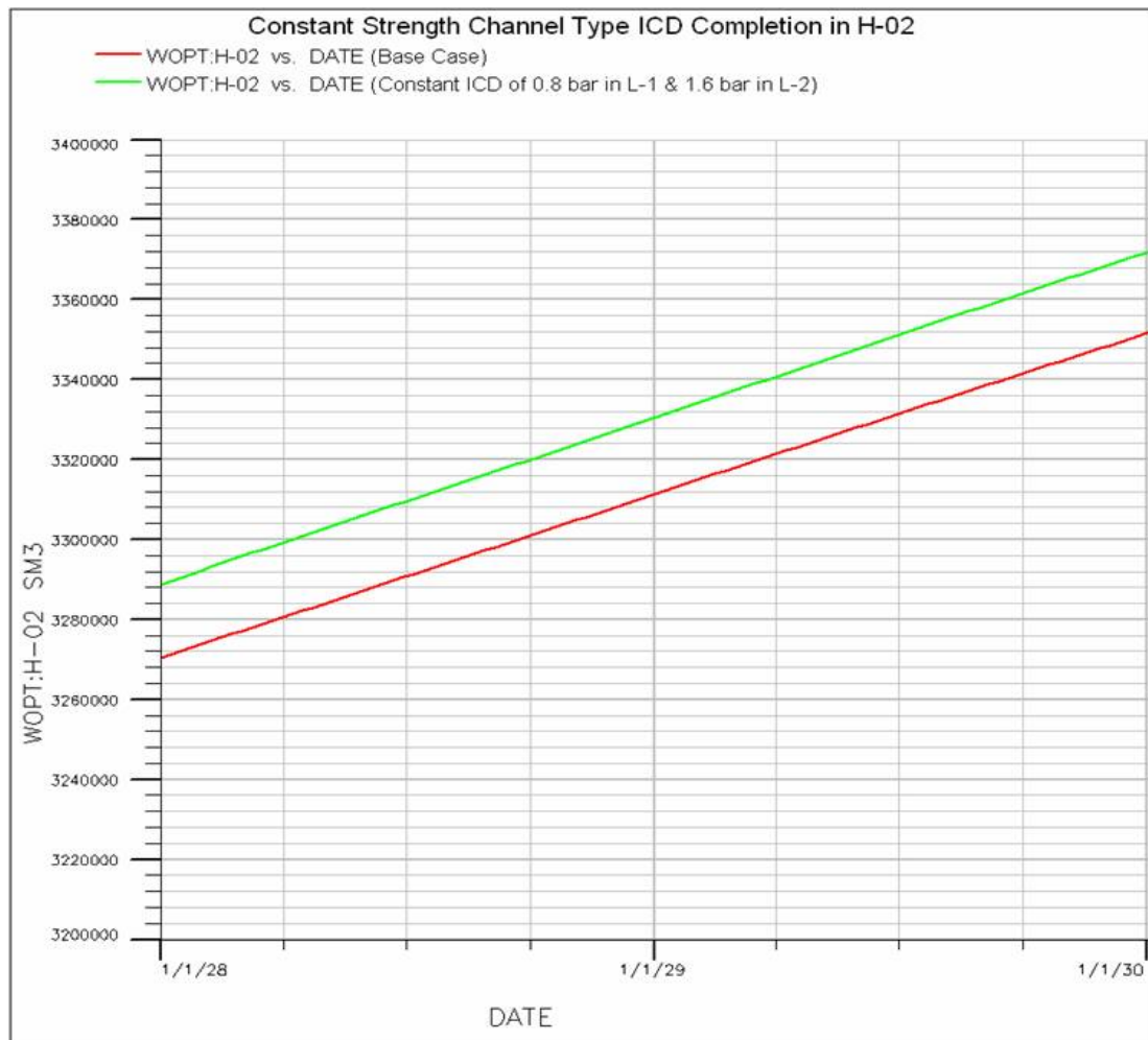
Figure 6-45: Comparison of the H-02 ICD and the base case completions
