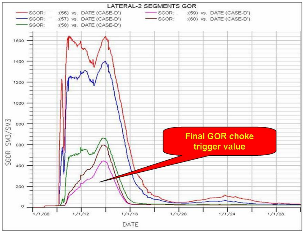
Figure 6-47: GOR performance of selected ICDs from well H-02, L-2 showing both high and low GOR segments
