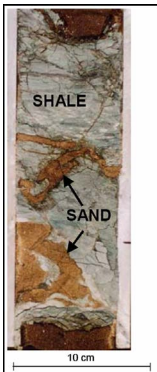
Figure 6-17: Core photo showing Lista shale with injection sands [236]
