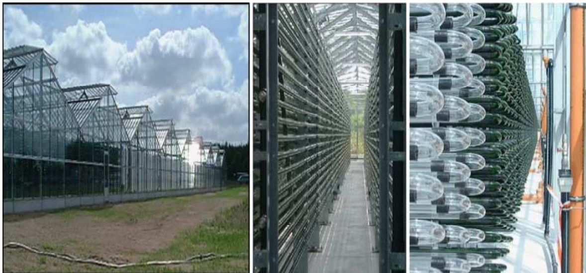
Figure 3.5 A high-end closed bioreactor system (Schenk et al., 2008).
