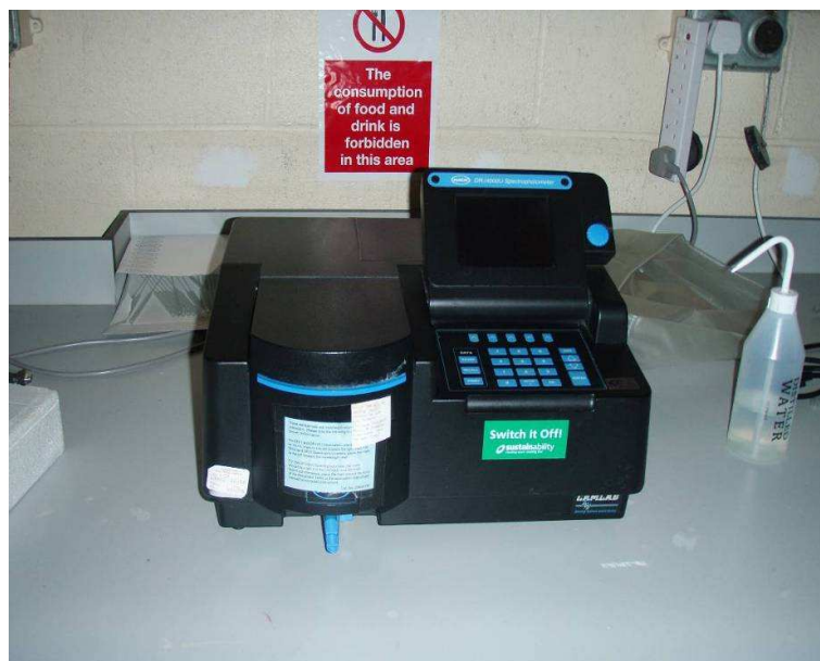
Figure 4.4 The spectrophotometer (CAMLAB DR/4000 U)
