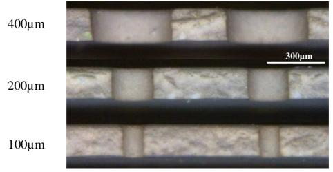
Figure 5.11: Cross section of vias showing the vertical walls obtained after 4 scans with a 400, 200 and 100µm apertures
