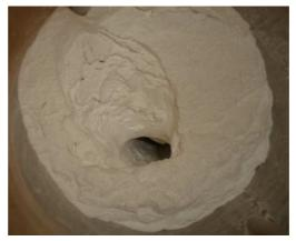
Figure 3.8: Typical example of a cavity formed inside the powder in the reservoir
