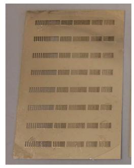
Figure 5.16: Nickel mask B featuring rectangular apertures
