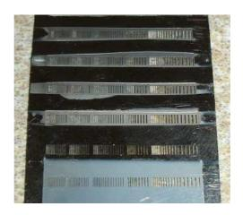
Figure 4.10: Photograph of a 100µm thick powder blasted mask featuring 6 sets of rectangular apertures 2mm long
