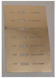
Figure 5.25: Nickel mask C featuring crosse and triangle shape
