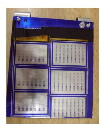
Figure 4.21: Complex pattern design created with 4 laminated dry film layers exposed at 3000mJ onto the stainless steel plate
