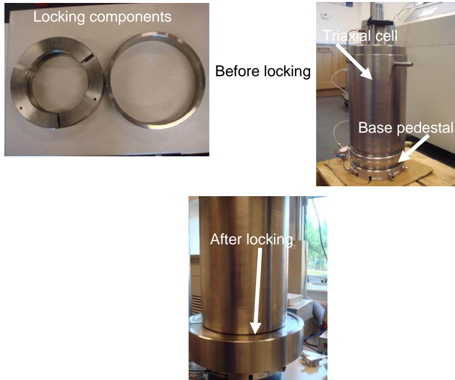
Figure 3.7 Locking system of the Triaxial cell to the base pedestal
