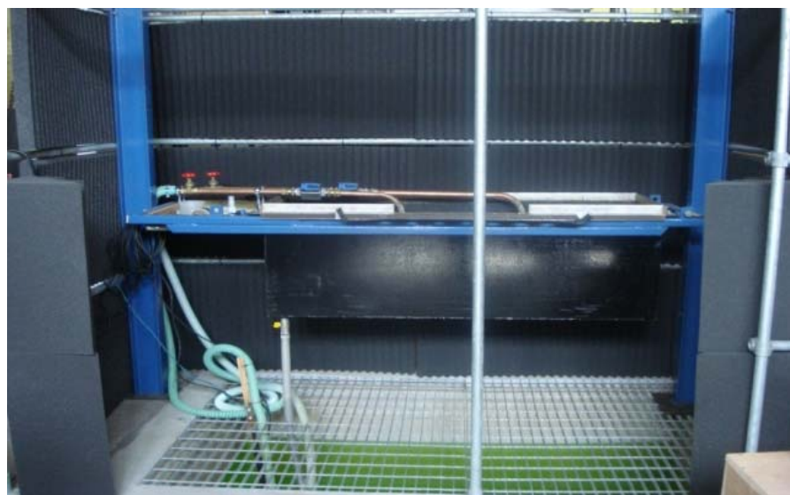
(b) Picture of test structure with tank fixed at 1.0 m (height of falling water).
