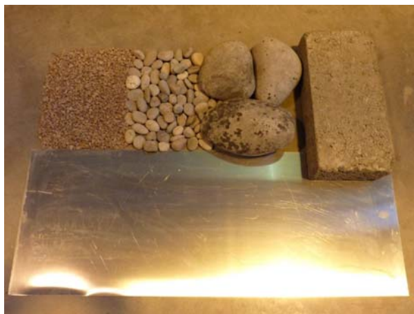
Figure 3.2 Impact materials used for tests, from top left to bottom right: gravel, pebbles, boulders, concrete block and metal plate.
