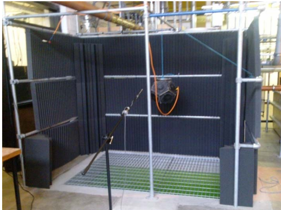
Figure 3.12 Test structure covered with absorption panels and bass traps, and sound source placed 1.2 m above the ground.
