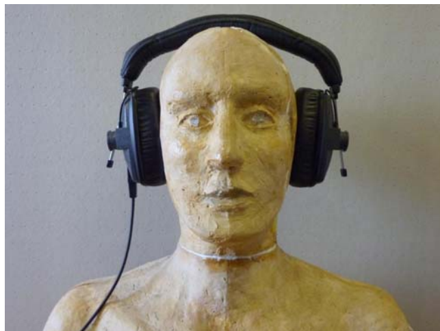
Figure 3.22 Setup used for the calibration of recorded signals.
