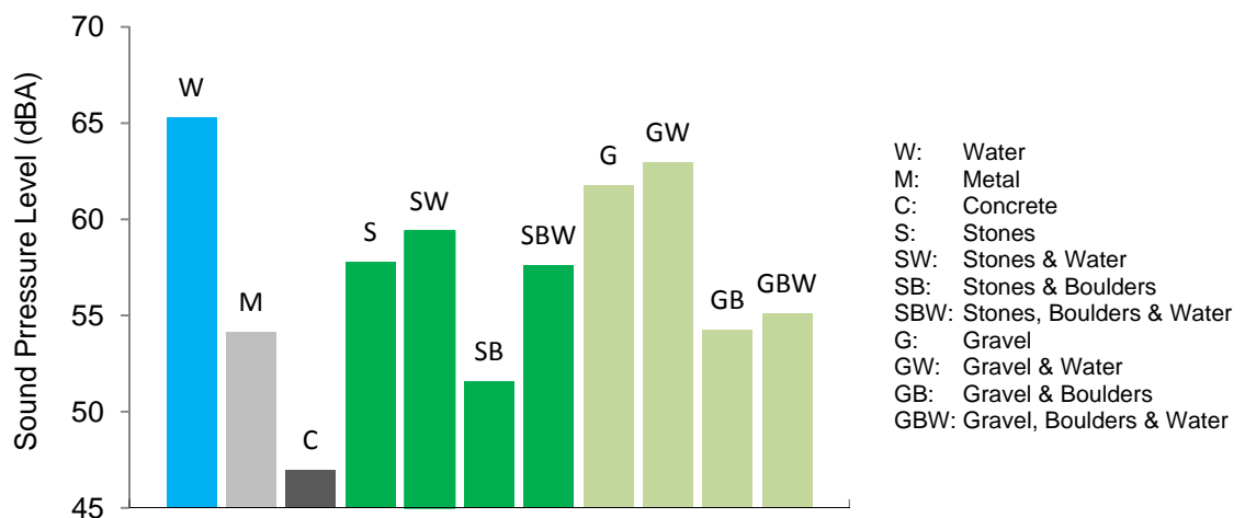
Figure 4.19 L_{Aeq} of waterfall plain edge 0.5 m height, 1 m width and 30 l/min, with different impact materials.
