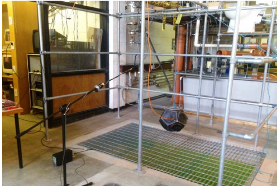
Figure 3.11 Setup used for reverberation time tests: no panels and omnidirectional sound source placed 0.5 m above the ground (with water inside the sump tank).
