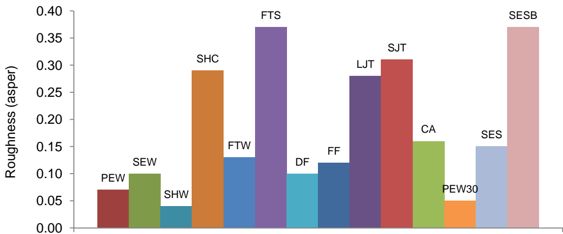
Figure 5.18 Roughness of water features measured in the laboratory.
