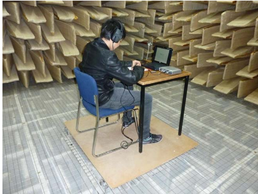
Figure 3.23 Auditory tests carried out in the anechoic chamber of Heriot-Watt University.
