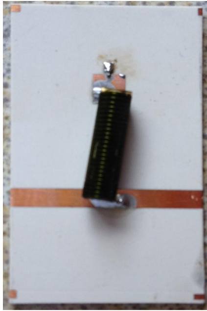
Fig 6. Photograph of Bias Network from Fig 3
