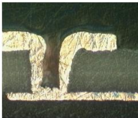
Figure 7. 75 micron via in LCP circuit.
