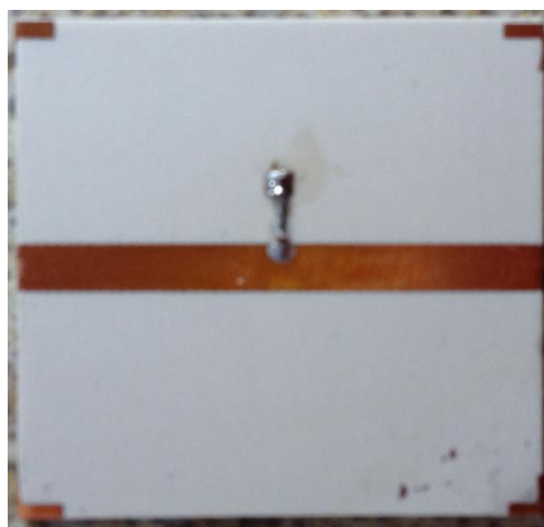
Fig 5. Photograph of Bias Network from Fig 2
