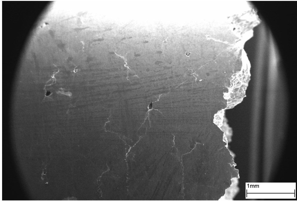
Figure III.3: Cracks starting from internal voids and pores near to the surface.
