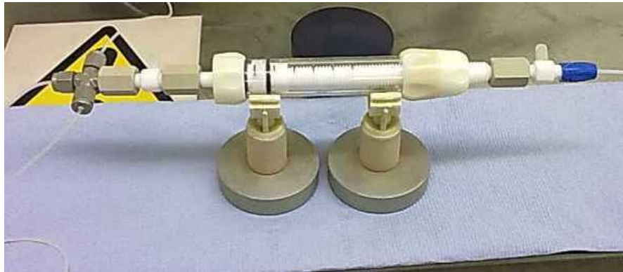
Figure 3.5: Column without sand for dead volume measurement
