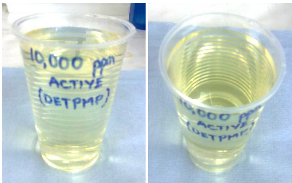
Figure 4.9: DETPMP in NFFW at 10,000ppm active. It is soluble at this concentration and yellowish in colour.
