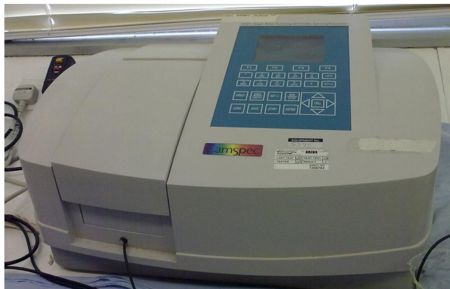
Figure C.3: UV/Vis Spectrophotometer - Camspec M302
