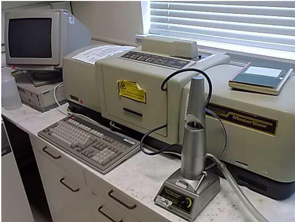
Figure C.4: Particle Size Analyzer - Malvern MS-20
