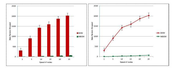
Figure 7.23: Data Dropped vs Speed of Nodes (Dynamic network: Pause Time 0 sec)
