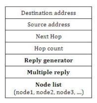
Figure 3.11: Route Reply packet structure of SMORT
