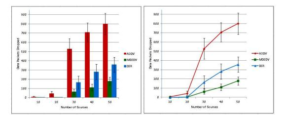
Figure 8.8: Data Dropped vs Number of Sources (Static network)
