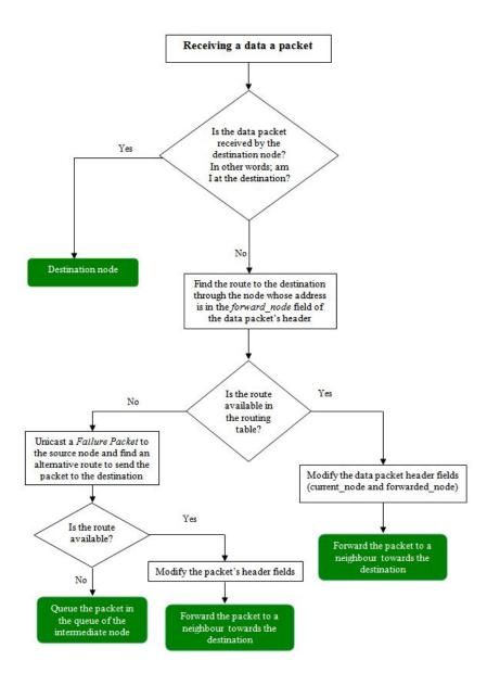
Figure 5.4: Receiving data packets Flowchart
