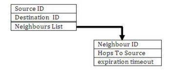
Figure 3.5: The Structure of each RREQ table entry in AODVM
