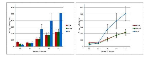
Figure 8.3: Average End to End Delay vs Number of Sources (Dynamic network)
