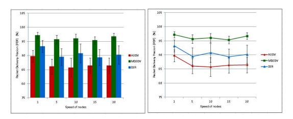
Figure 8.26: PDF vs Speed of Nodes (Static network)
