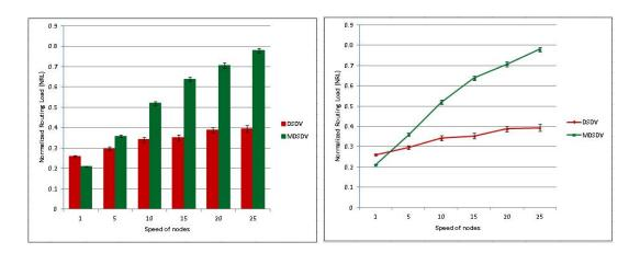
Figure 7.21: NRL vs Speed of Nodes (Dynamic network: Pause Time = 0 sec)
