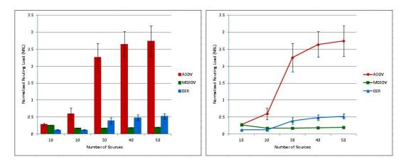
Figure 8.6: NRL vs Number of Sources (Static network)
