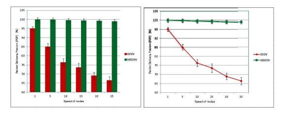
**Figure 7.17:** PDF vs Speed of Nodes (Dynamic network: Pause Time = 0 sec)
