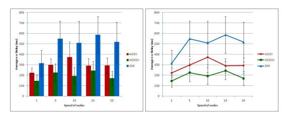
Figure 8.28: Average End to End Delay vs Speed of Nodes (Static network)
