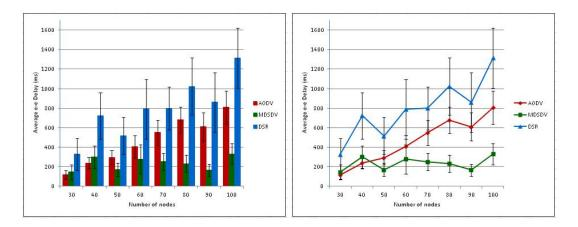
Figure 8.12: Average End-to-End Delay vs Number of Nodes (Static network)
