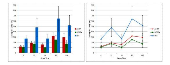
Figure 8.20: Average End to End Delay vs Pause Time (High Speed)
