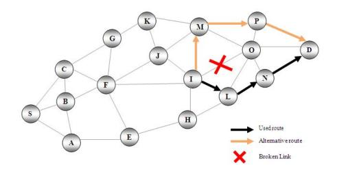
Figure 5.2: Node I is using an alternative route to forward data
