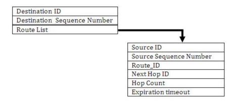
Figure 3.6: The Structure of each Routing table entry in AODVM
