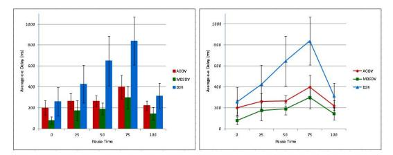
Figure 8.19: Average End to End Delay vs Pause Time (Low Speed)
