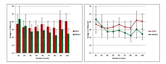
Figure 7.4: Average End to End Delay vs Number of Nodes (Pause Time 200 sec)
