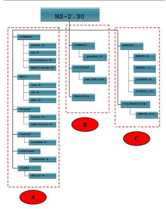
Figure 4.2: MDSDV Modules: Unmodified (A), Modified (B) and New (C)
