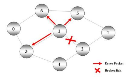
Figure 5.12: Node 1 discovers a broken link and broadcasts an Error Packet
