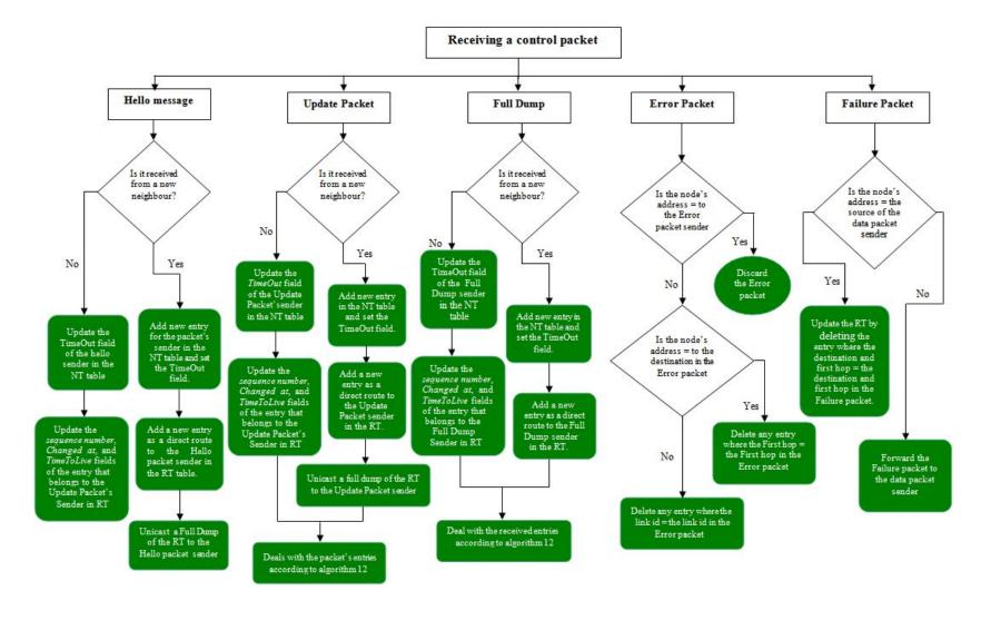
Figure 5.6: Receiving Control Packets Flowchart
