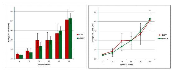
Figure 7.19: Average End to End Delay vs Speed of Nodes (Dynamic network)
