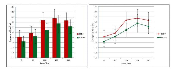
Figure 7.11: Average End-to-End Delay vs Pause Time (Low speed: 1 m/sec)
