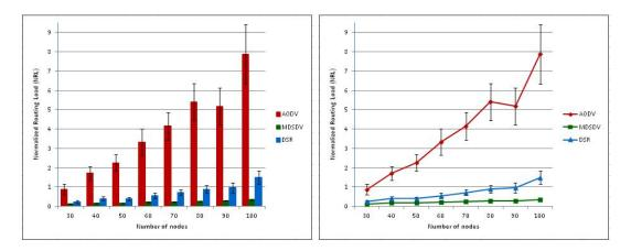
Figure 8.14: NRL vs Number of Nodes (Static network
