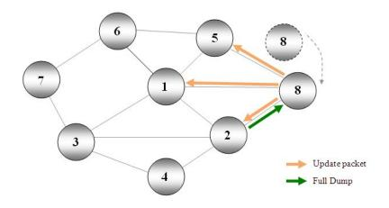
Figure 5.10: Node 8 is broadcasting an Update Packet and receiving a Full Dump
