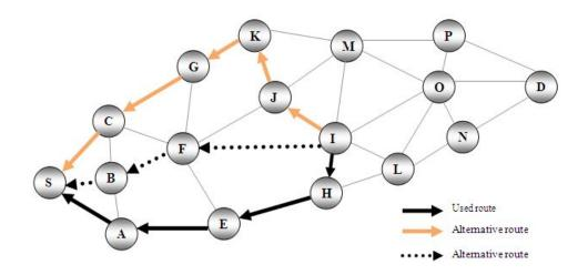
Figure 5.3: Node I is unicasting a *Failure Packet* to the source node (Node S)
