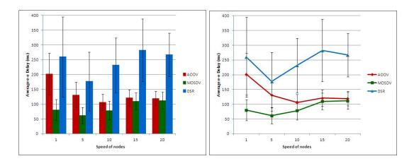
Figure 8.27: Average End to End Delay vs Speed of Nodes (Dynamic network)
