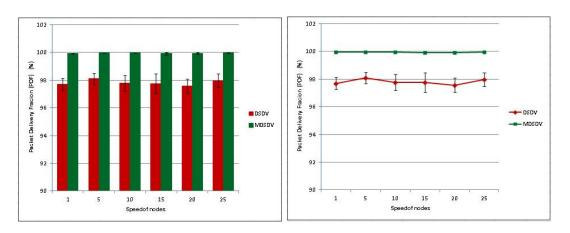
Figure 7.18: PDF vs Speed of Nodes (Static network: Pause Time = 200 sec)
