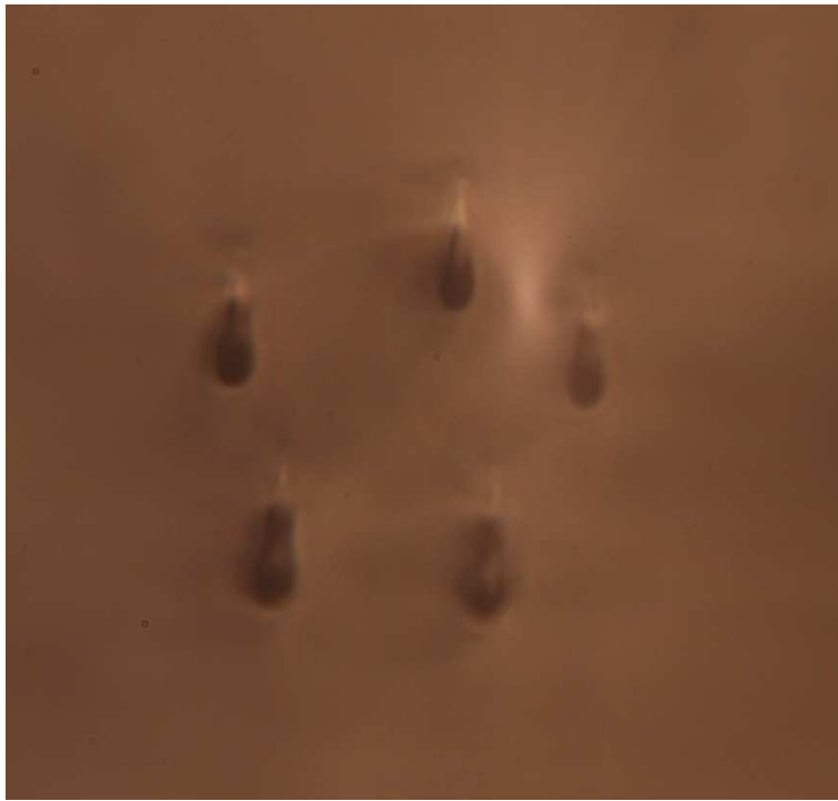
Figure 7.5. Microscope image of one of the cladding written waveguides inscribed in N-SSK5.
