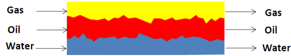
Figure 4-1: Steady-state coreflood experiment for determining relative permeability. The fluid proportions produced at the outlet are equal to the proportions injected at the inlet.
