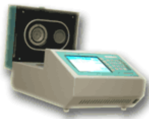
Figure 3.4 A picture of the LabMaster- a_w used in this work for measuring water activity of aqueous phase
