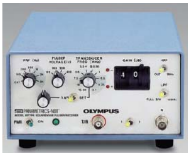
Figure 2.7 Picture of Panametrics 5077PR pulser-receiver
