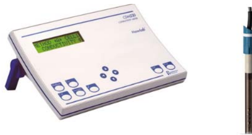
Figure 2.6 Picture of conductivity meter and conductivity cell
