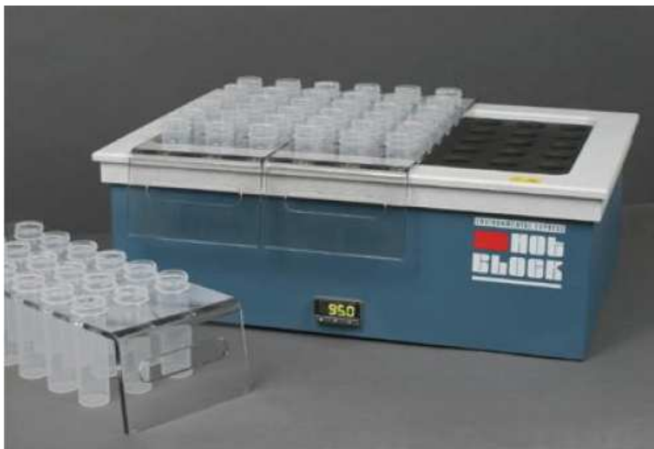
Figure B1: Electric water bath to heat sediment samples followed by acid digestion.
