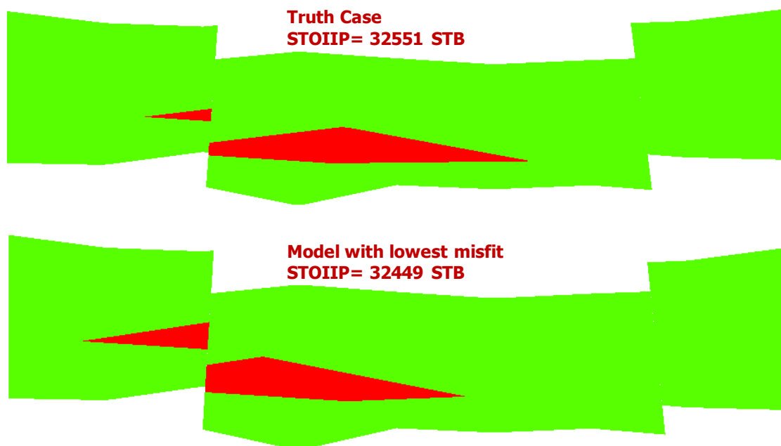
Figure 6.24: Maximum likelihood model vs. truth case for uncertain faults and pinchout
