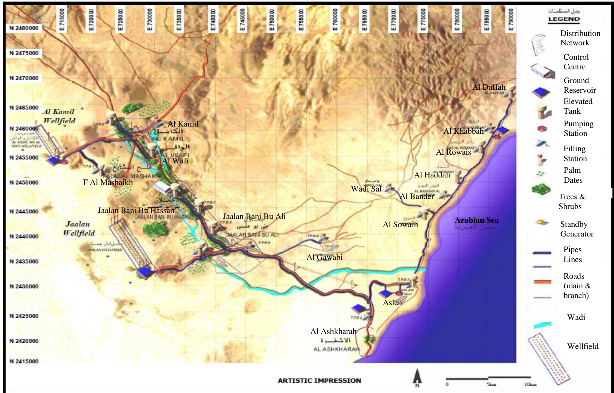
Figure 4.5: Map showing the main components of the Ash Sharqiyah Sands Groundwater Scheme (Dr. Ahmed Abdel Warith & Partners LLC, 1999)
