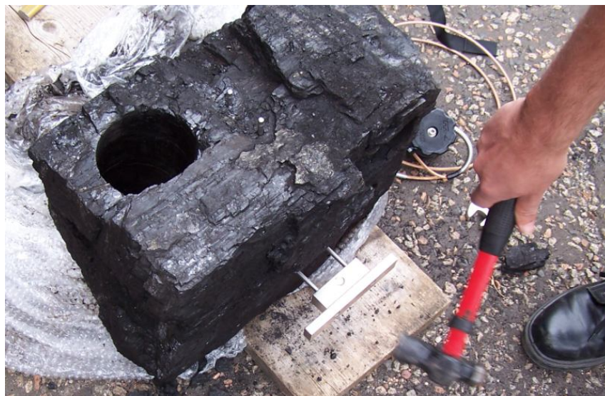
Figure 28 – The second step of probes' introduction consists in hammering the probes within the drilled holes. Many blocks disintegrated during this process.
