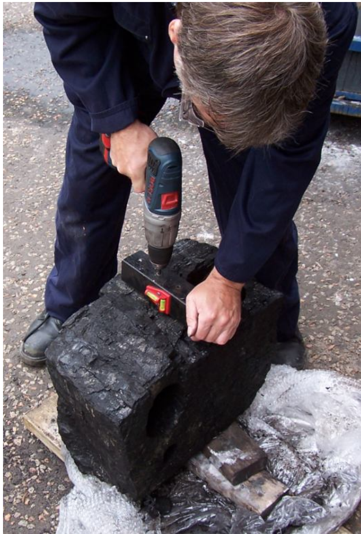
Figure 27 – The first step of probe insertion consists of drilling the holes. In this picture, the coal block is not encased in its concrete case because its dimensions exceeded the mould size.
