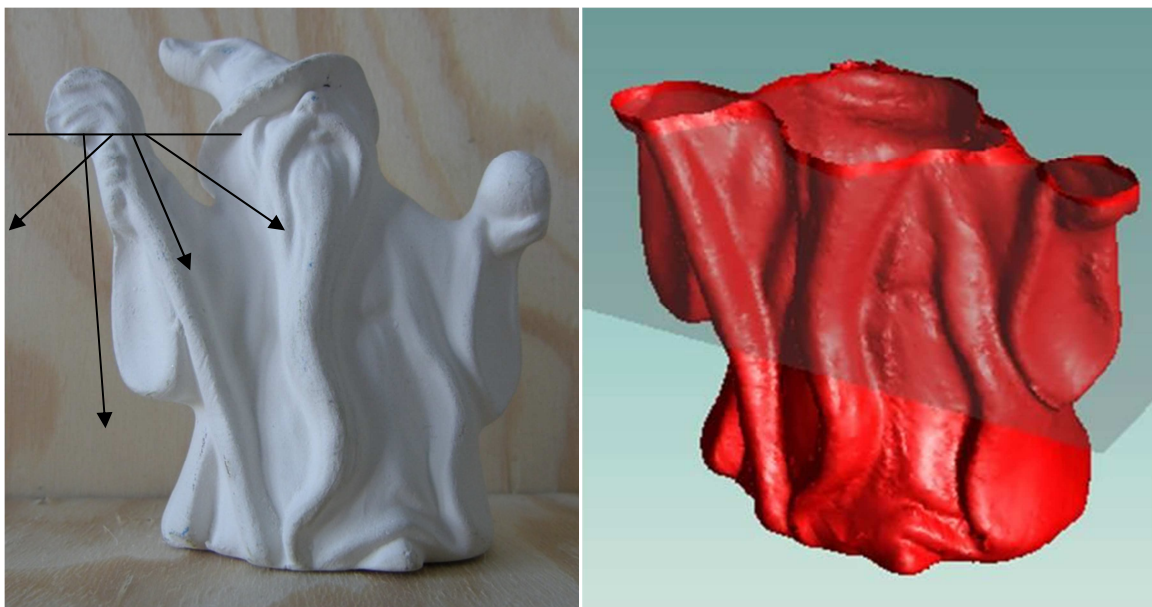
Figure 1-2 Complex model with linear slice produces significantly different normal vectors
