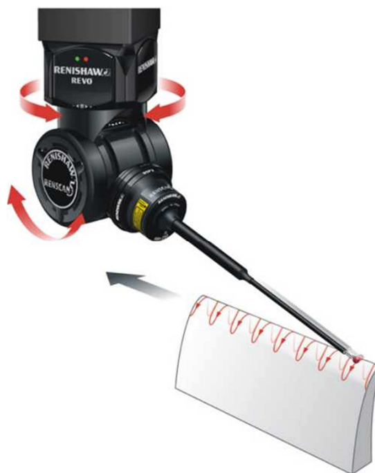
Figure 1-6 Blade sharp edge sweep scan (13)
