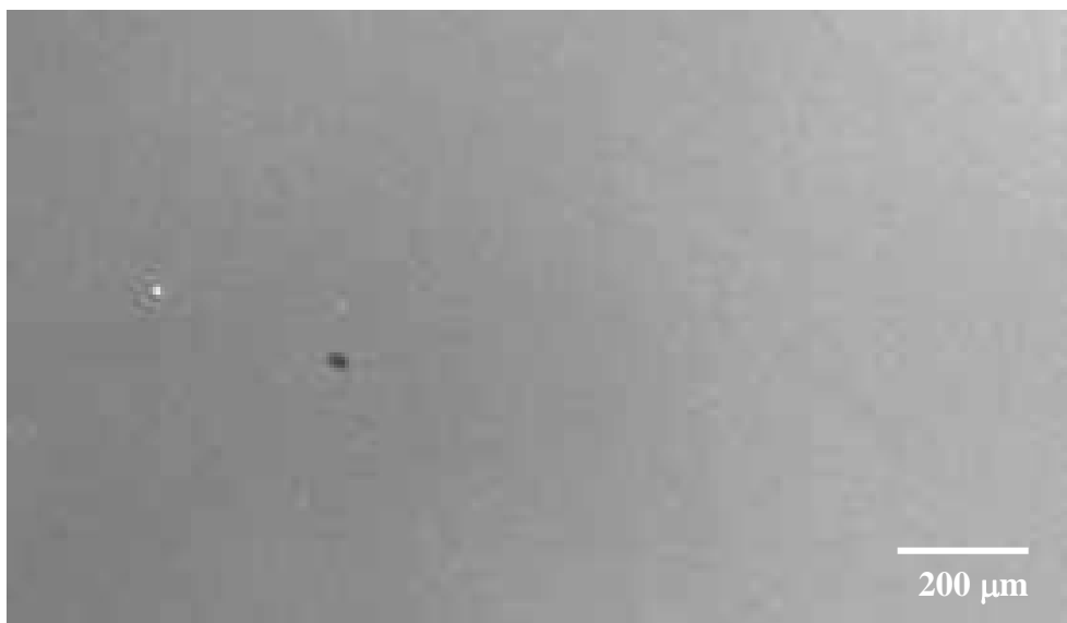
Figure 8-8 Represents the surface condition of a control specimen without treated with acid HCl
