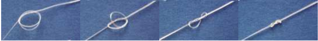
Figure 2.4 A fiber of a thermoplastic SMP was stretched and formed a loose knot, both ends of the suture were fixed. The photos shows how the knot tightened in 20 s when heated to 40°C [65].
