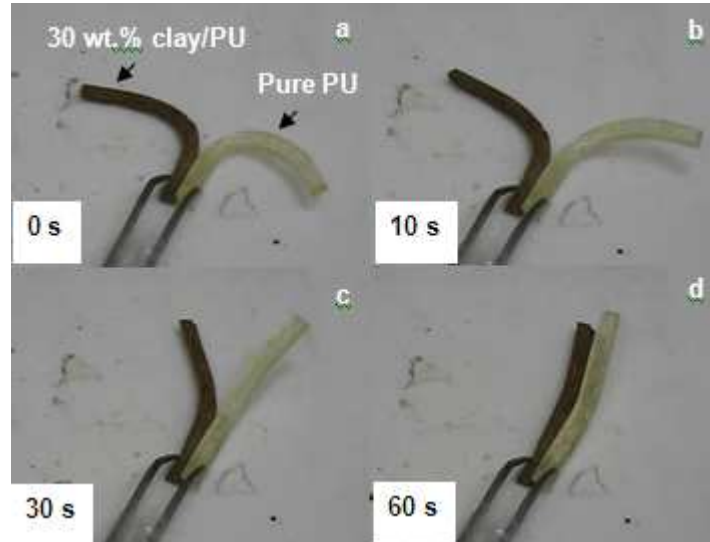
Figure 4.15 Recoveries of shape memory samples heated on a hotplate with a surface temperature of 80 °C.
