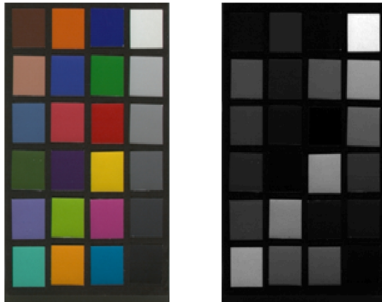
Figure 4.21: MacBeth colour chart used in the dispersion simulation. Colour image and gray-scale image at 550nm.
