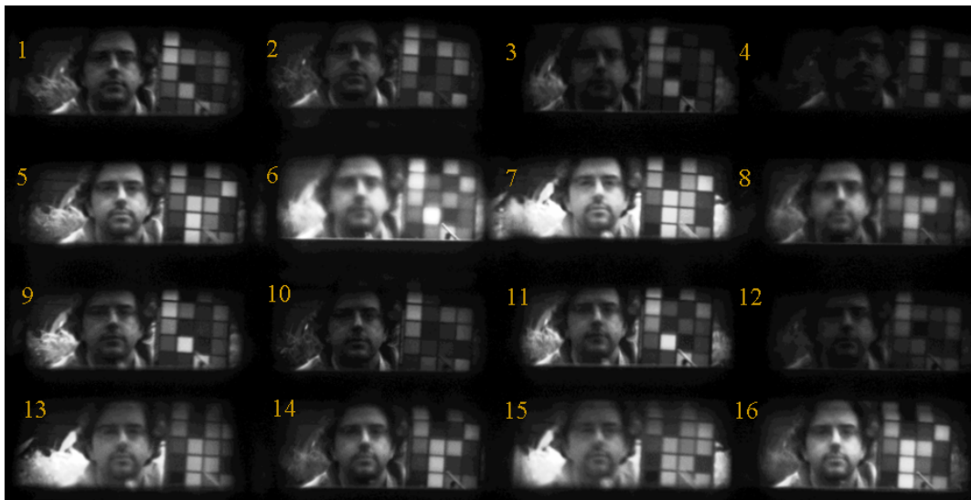
Figure 4.18: Image from 16-channel system with filter array and array of corrective glass tiles.
