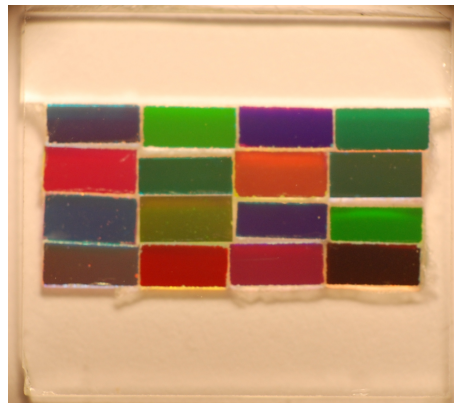
Figure 4.14: Photograph of the filter array.
