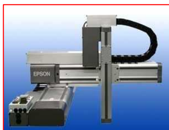
(a) PPP Serial Rigid-Body Manipulator (Source: www.directindustry.com)
