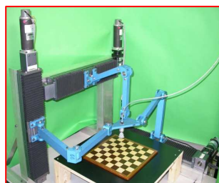
(b) 3-PRRR Parallel Rigid-Body Manipulator (Gosselin and Kong, U.S. Patent 2004, Courtesy of Gosselin, Uni. Laval)
