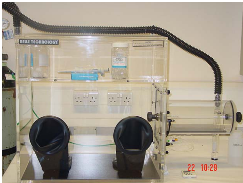
Figure 3.1 Nitrogen glove box where all the sulphide studies are performed.
