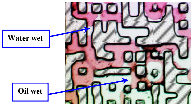
Figure 3-7: The same section of the micromodel as Figure 6 after CWI, which shows two types of wettability in the micromodel, Preliminary Experiment No.2 (red oil and clear water were used).
