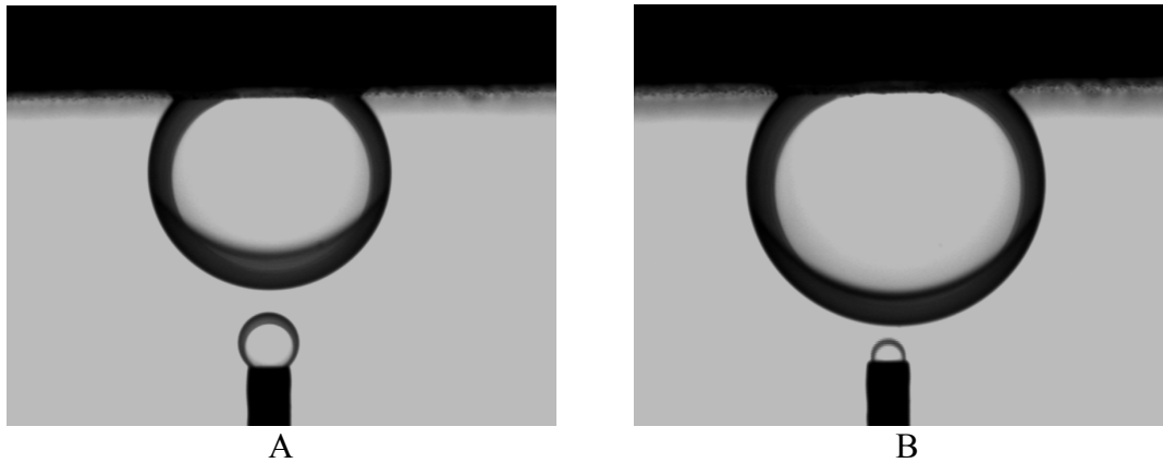
Figure 5-22: Effect of oil droplet size on the contact angle in brine/n-decane/quartz system at P=1627 psi, T=58 °C, when oil droplet size is A) 11.23 \mu\text{L} , BCD=0.2244 cm, \theta=49.5 and B) 21.13 \mu\text{L} , BCD=0.2818 cm, \theta=49.0 .
