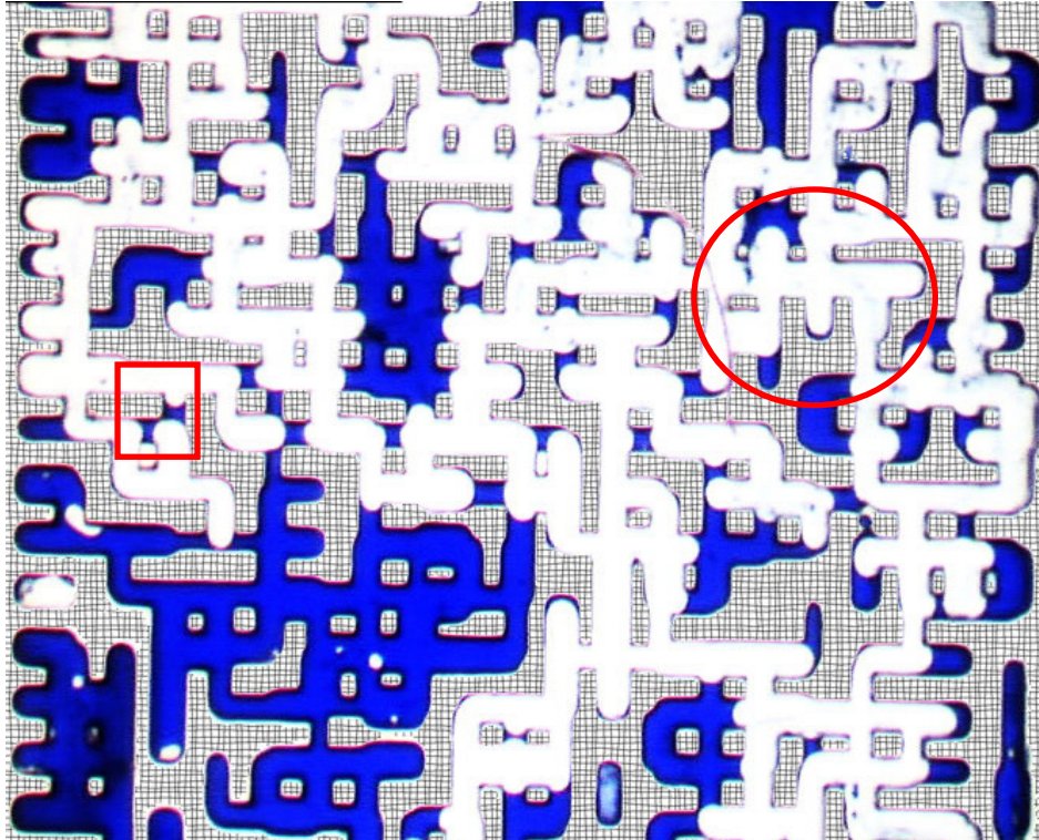
Figure 3-10: Initial oil saturation in Experiment No.1 (Tertiary CWI- Decane) after the first drainage stage.
