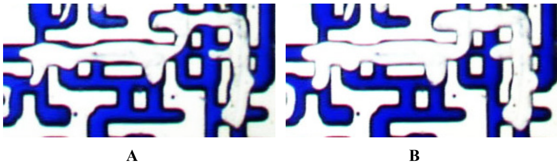
Figure 3-32: An oil ganglion in Experiment No.3 (Tertiary CWI- Viscous oil): A) after the 1 st WI; B) swollen oil at the end of the 1 st CWI stage.
