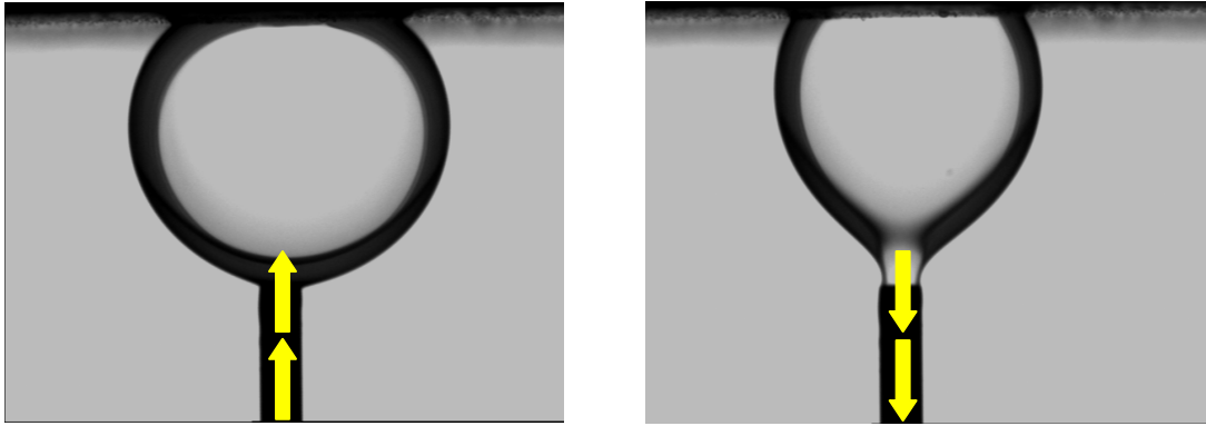
Figure 5-24: The position of an oil droplet and the needle to measure advancing (left hand side) and receding (right hand side) contact angles in a quartz/brine/n-decane system at 1627 psi and 58 °C.
