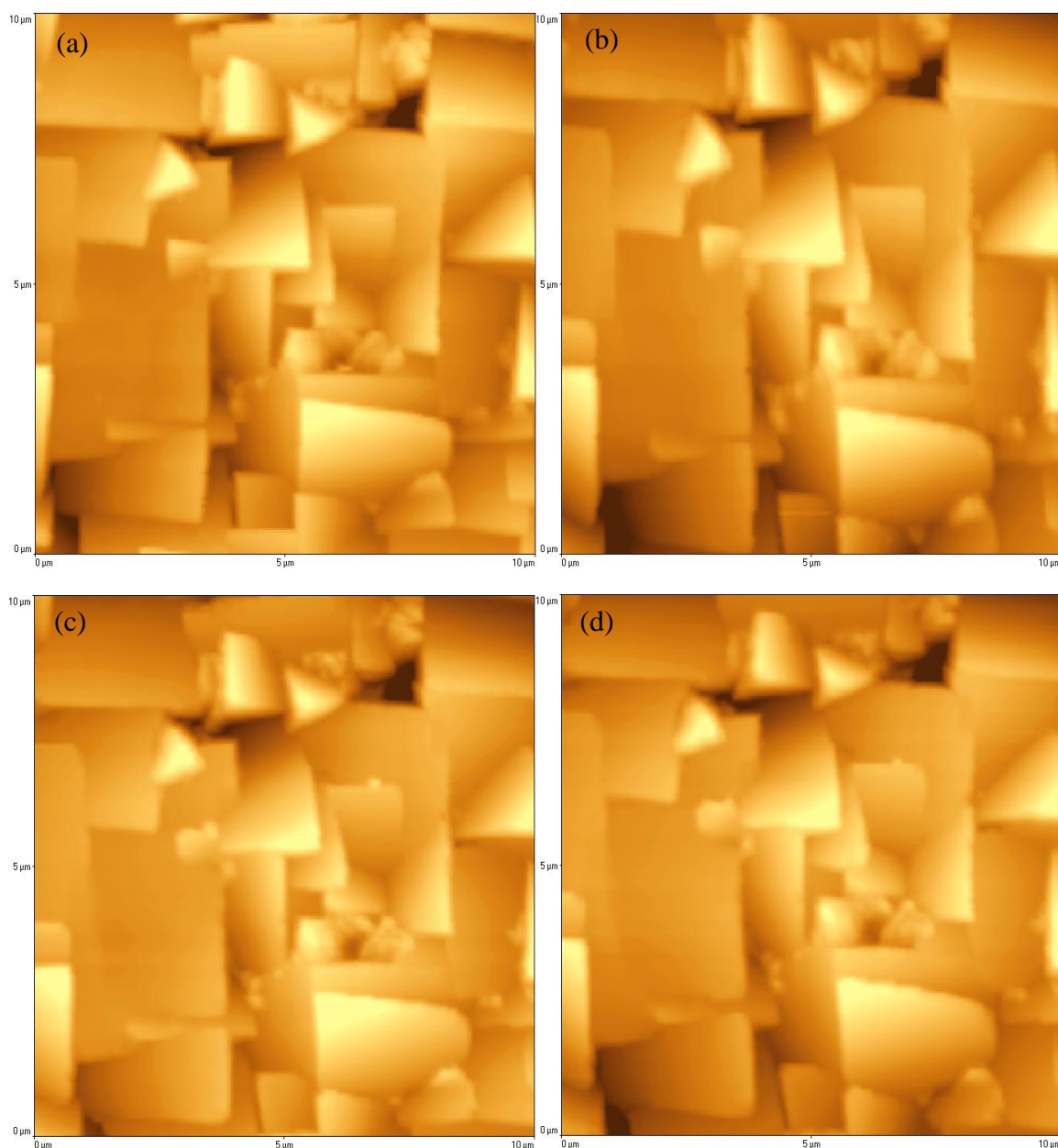
Figure 4.10 AFM images of the same (100) highly oriented CVD diamond crystallites after successive microwave-assisted hydrogen plasma treatments. (a) as-grown film, (b) 8 hours, (c) 16 hours and (d) 20 hours.
