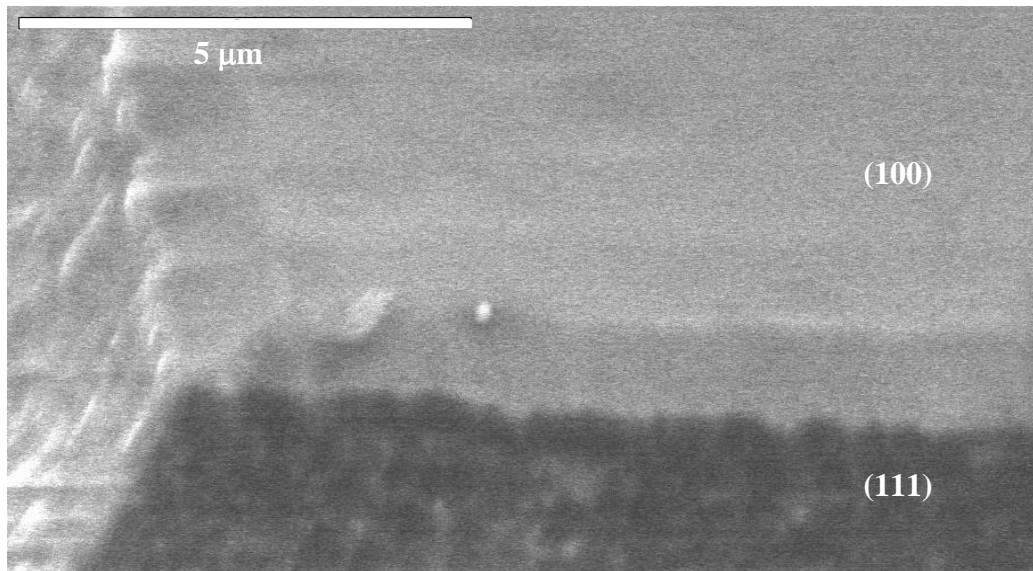
Figure 6.12 SEM image of the (100) and (111) diamond facets of a thermally oxidised CVD cubo-octahedral crystallite at 565°C and 1 atm pressure of dry O 2 for 9 hours.
