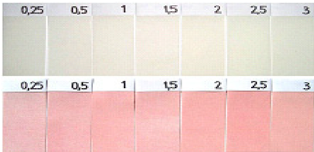
Fig. 4.1.3: Reflectance curves and photographs before and after irradiation of pigment P3 at different concentrations
