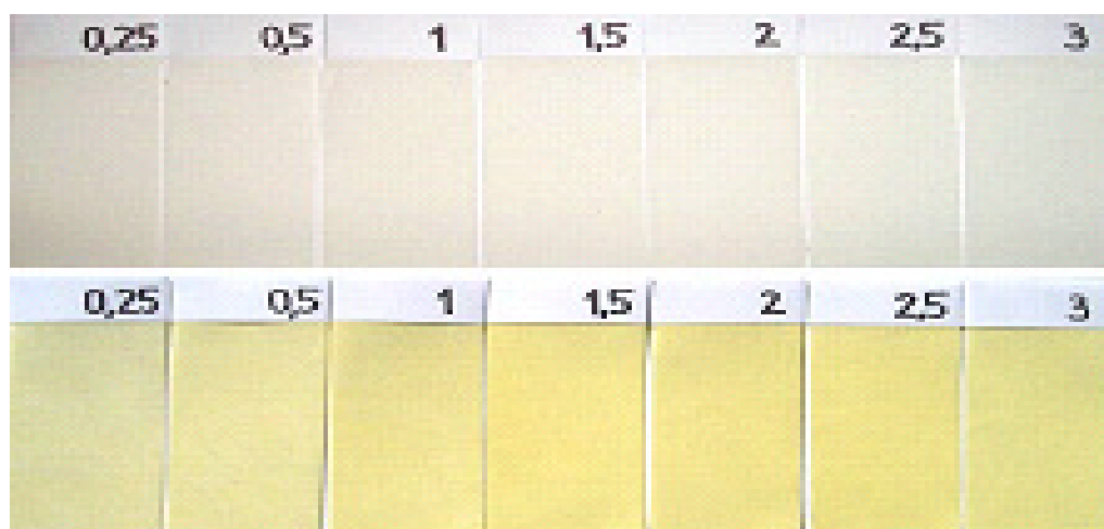
Fig. 4.1.5: Reflectance curves and photographs before and after irradiation of pigment P5 at different concentrations
