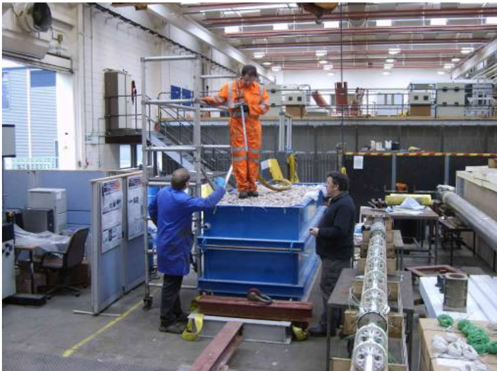
Figure 5.1. Application of the polymer to form XiTRACK within GRAFT
