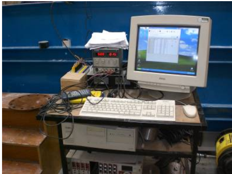
Figure 3.7. GRAFT data acquisition system, signal condition equipment and terminal board
