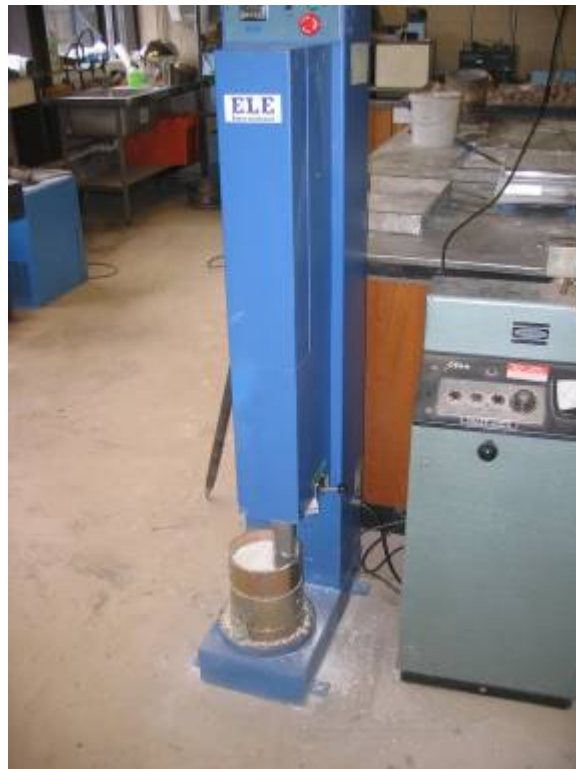
Figure 3.13. Automatic compactor and CBR mould
