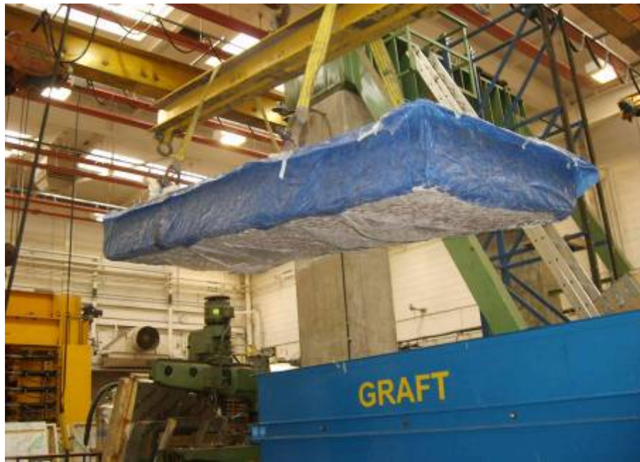
Figure 5.7. XiTRACK removal after 500,000 load cycles
