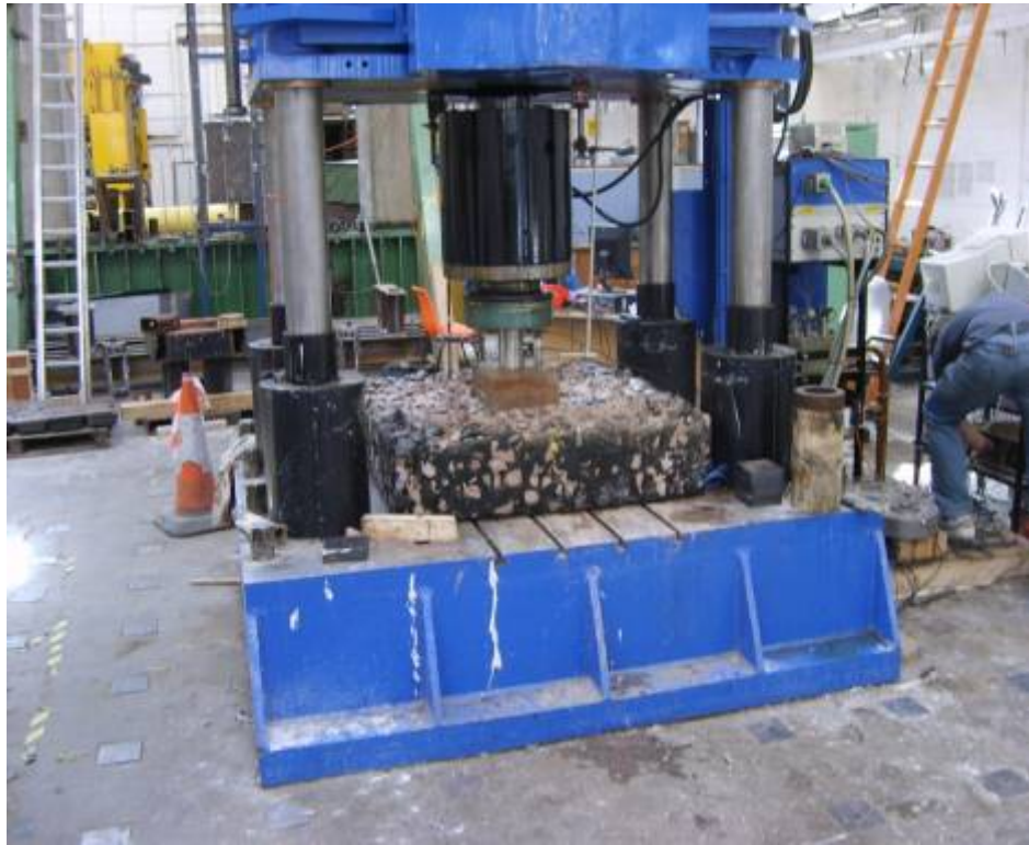
Figure 5.10. XiTRACK slab section under load
