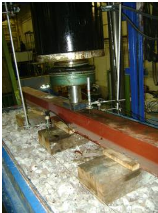
Figure 3.29. Track under loading - after validation tests (3 sleepers bolted to rail)
