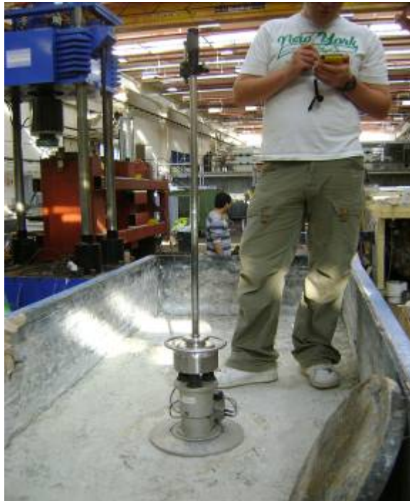
Figure 6.6. LFWD test in GRAFT
