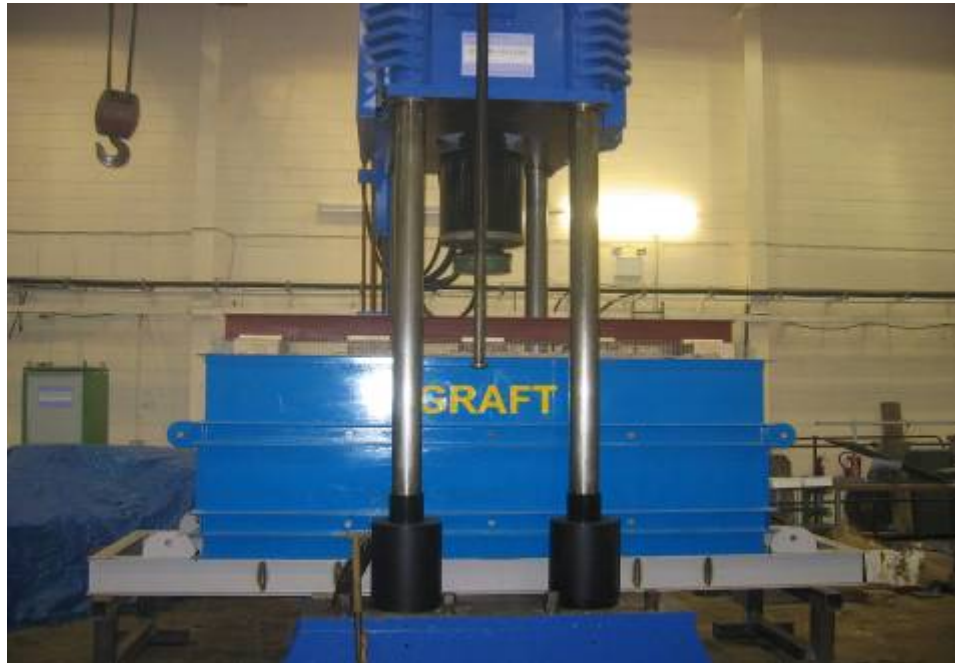
Figure 3.24. GRAFT facility ready for loading prior to initial validation tests (5 sleepers)
