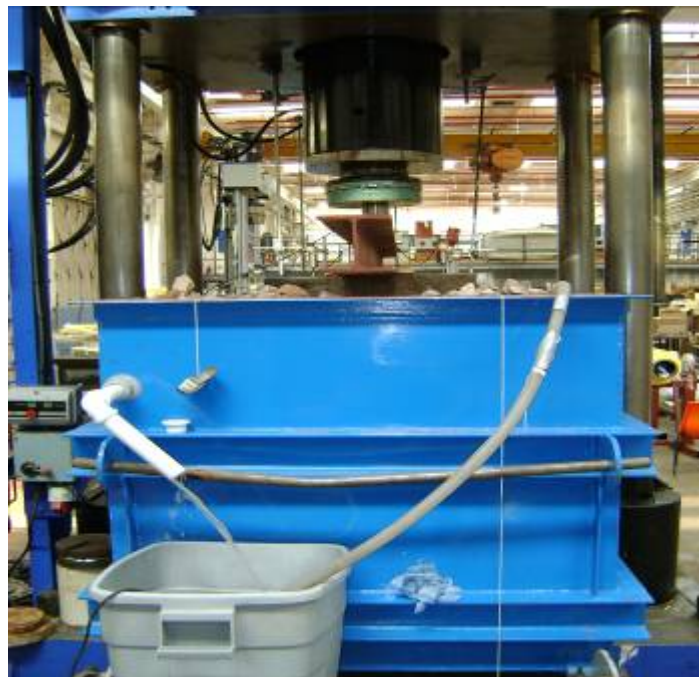
Figure 5.31. Water draining out the side of GRAFT 50mm above the top of the formation layer
