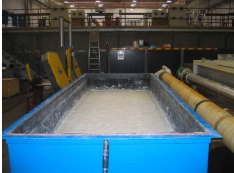
Figure 3.22. Initial track compacted Kaolin clay formation
