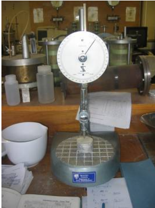
Figure 3.11. Cone penetrometer test undertaken on Kaolin clay
