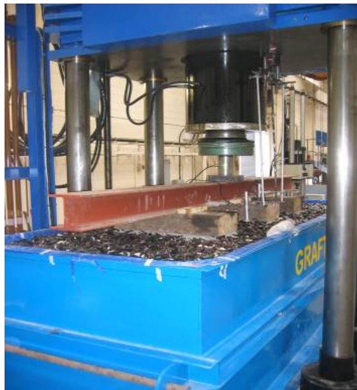
Figure 5.3. XiTRACK reinforcement under test in GRAFT
