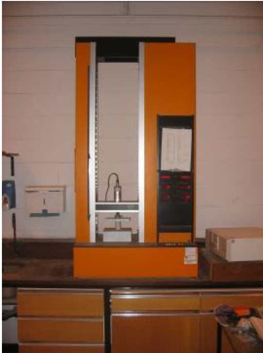
Figure 3.18. Typical unconfined compression test on clay sample
