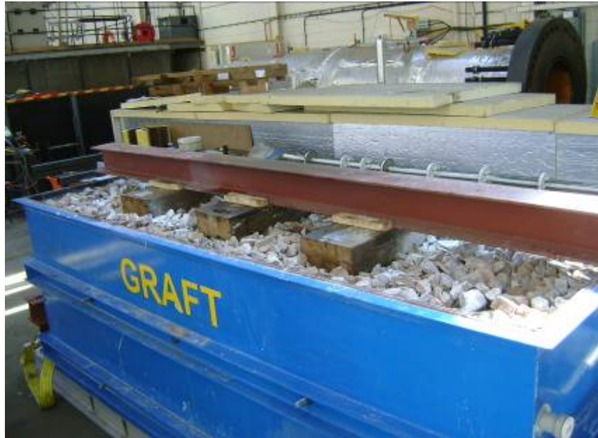
Figure 3.28. Fully constructed track prior to loading - after validation tests (3 sleepers)
