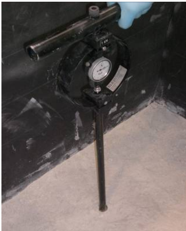
Figure 6.10. Proving ring penetrometer measurement in GRAFT
