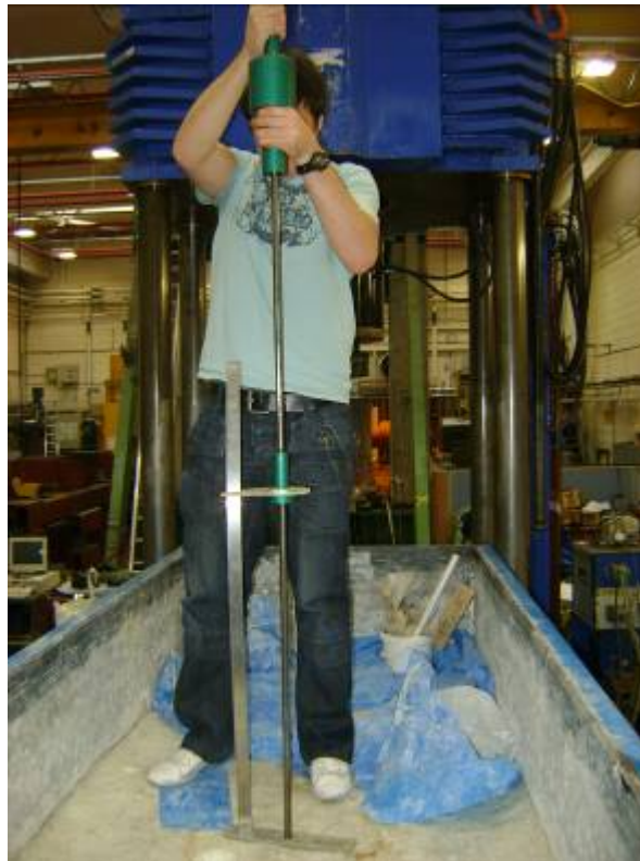
Figure 6.2. DCP test in GRAFT
