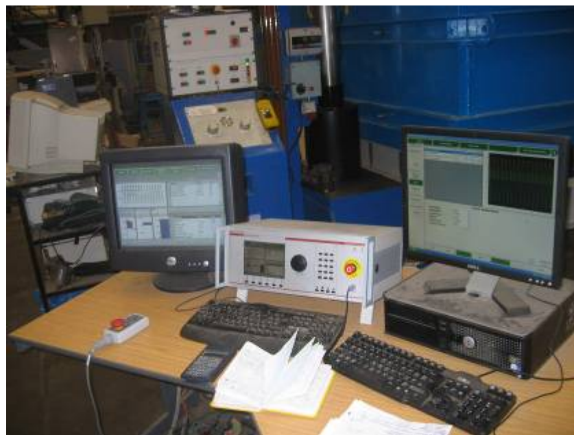
Figure 3.4. LOS machine controller and host computer
