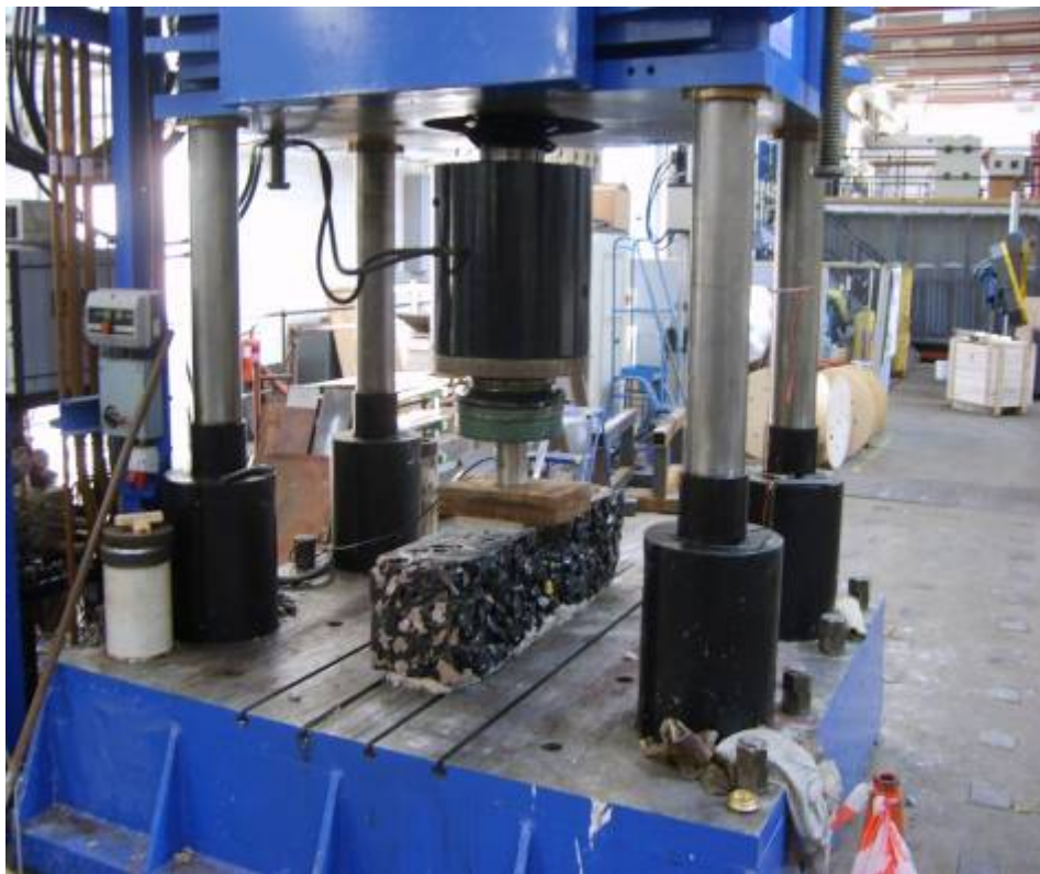
Figure 5.14. XiTRACK beam section under load
