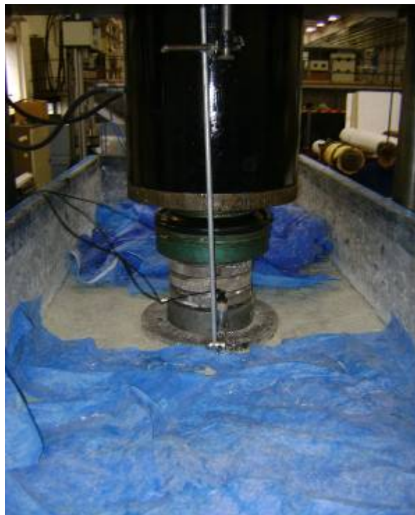
Figure 3.20. Typical plate load test undertaken in GRAFT
