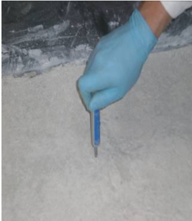
Figure 6.9. Pocket penetrometer measurement in GRAFT
