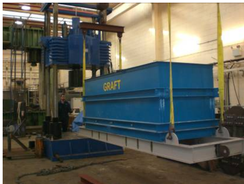
Figure 3.3. Steel tank to hold track being lifted into position under loading actuator
