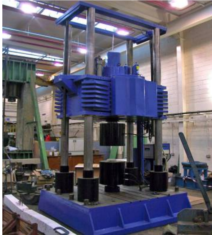
Figure 3.1. LOS hydraulic cyclic testing machine in the heavy structures lab
