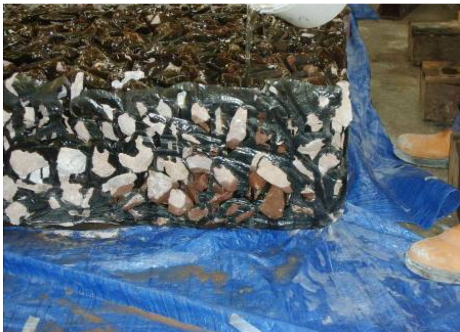
Figure 5.8. XiTRACK sample still free draining after 500,000 load Cycles
