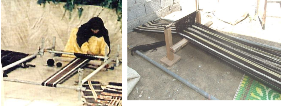
Figure 3:23 The use of metal piping as a basic structure for the ground loom. Photographed in Sowaiq, 2008
