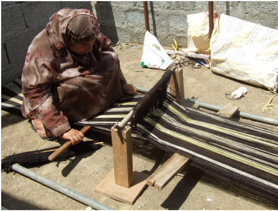
Figure 3:30 The weaver sit on the woven part to continue the weaving process, on her right is the stick shuttle and using the sword to beat the weft threads. Photographed in Sowaiq, 2008
