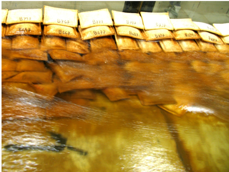
(c) Displacement due to (i) pressure differences between the main and void flow and (ii) sliding
