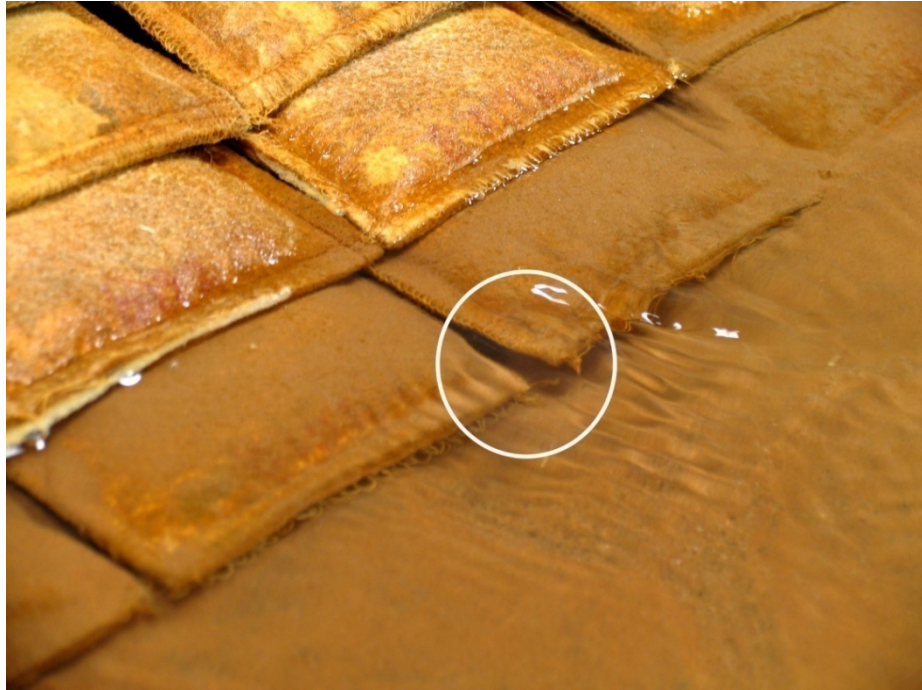
(a) Displacement due to (i) pressure differences between the main and void flow and (ii) toe scouring
