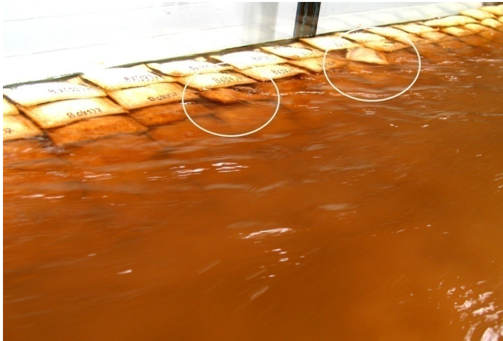
(c) Uplifting and sliding
