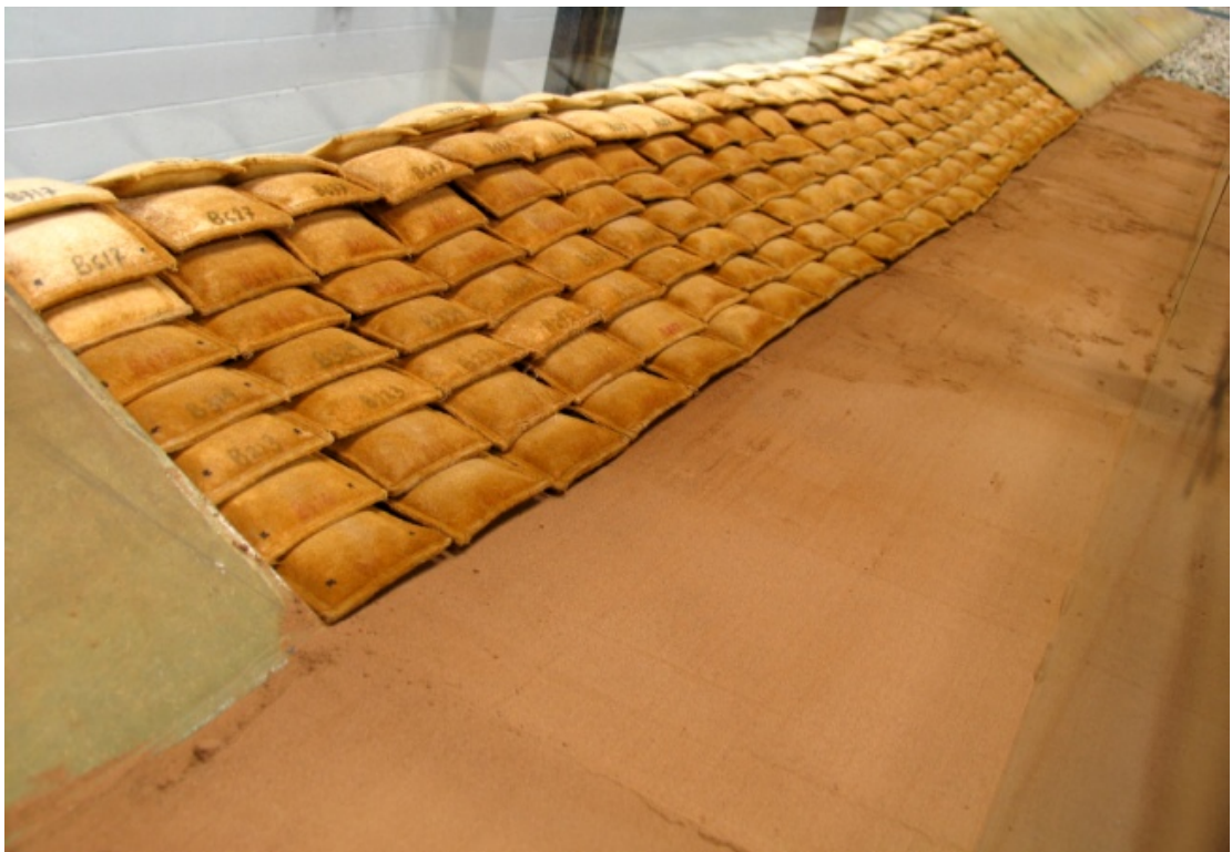
(b) Geobag revetment on sandbed
