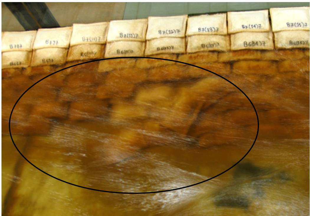
(b) Sliding, partial uplift and pullout
