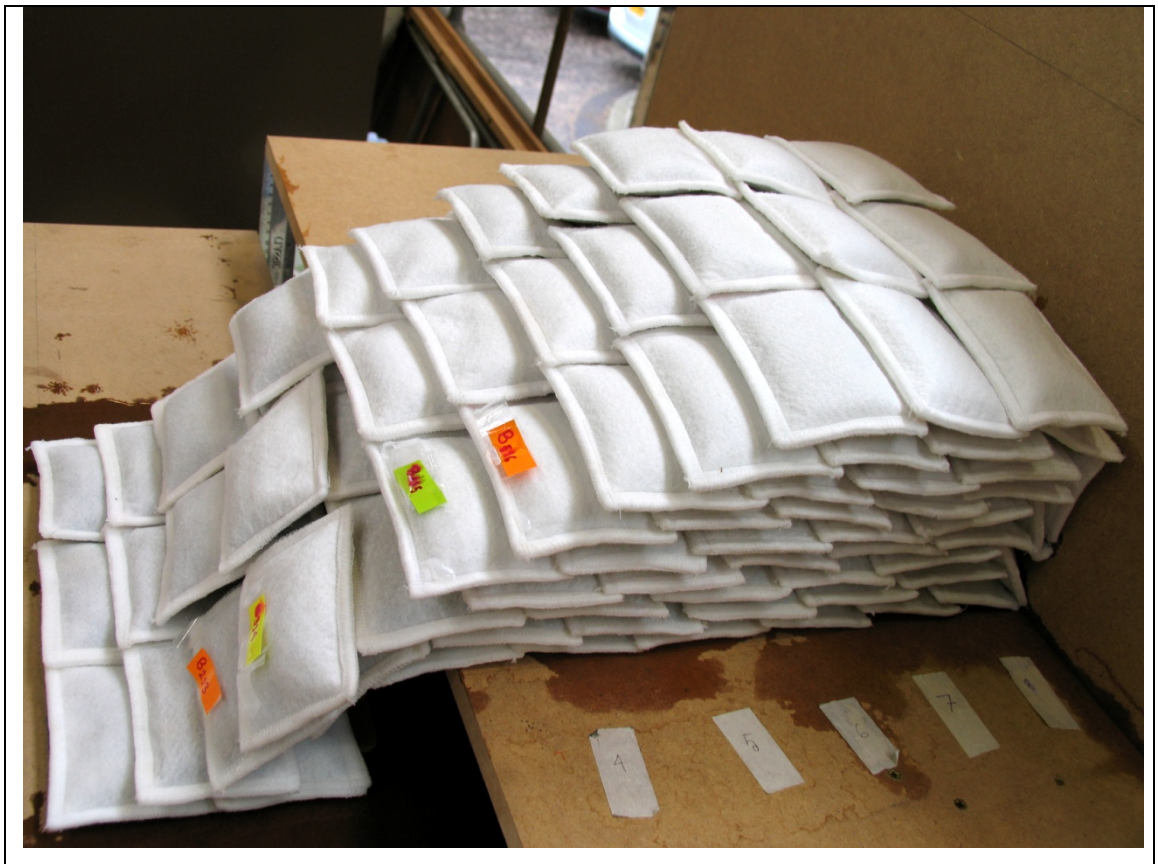
(c) Failure mode at 0.10 m scour depth in wooden test rig using Soaked bags
