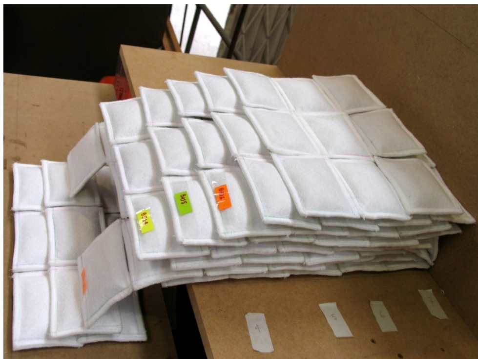
(b) Failure mode at 0.10 m scour depth in wooden test rig using dry bags
