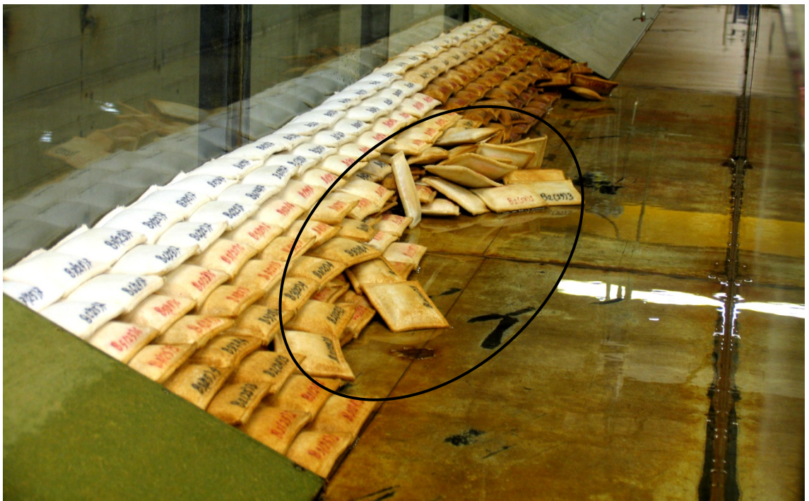
(b) Sliding zone (with slumps)
