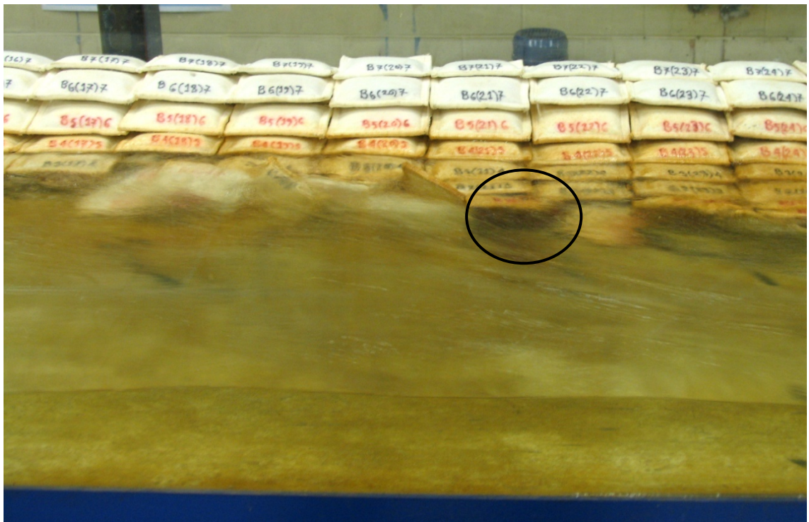
(a) Displacement due to (i) pressure differences between the main and void flow and (ii) uplift
