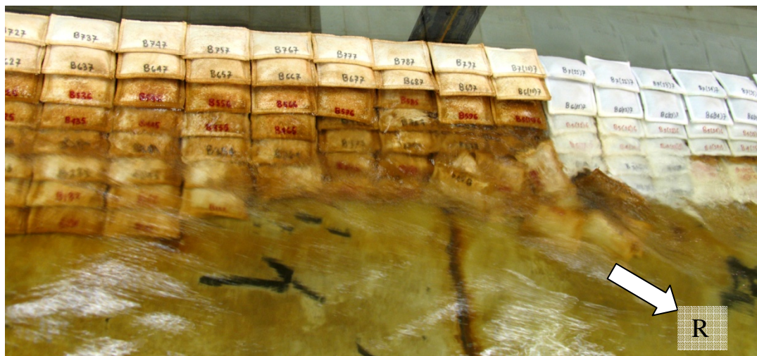
(a) Force causing geobag movement
