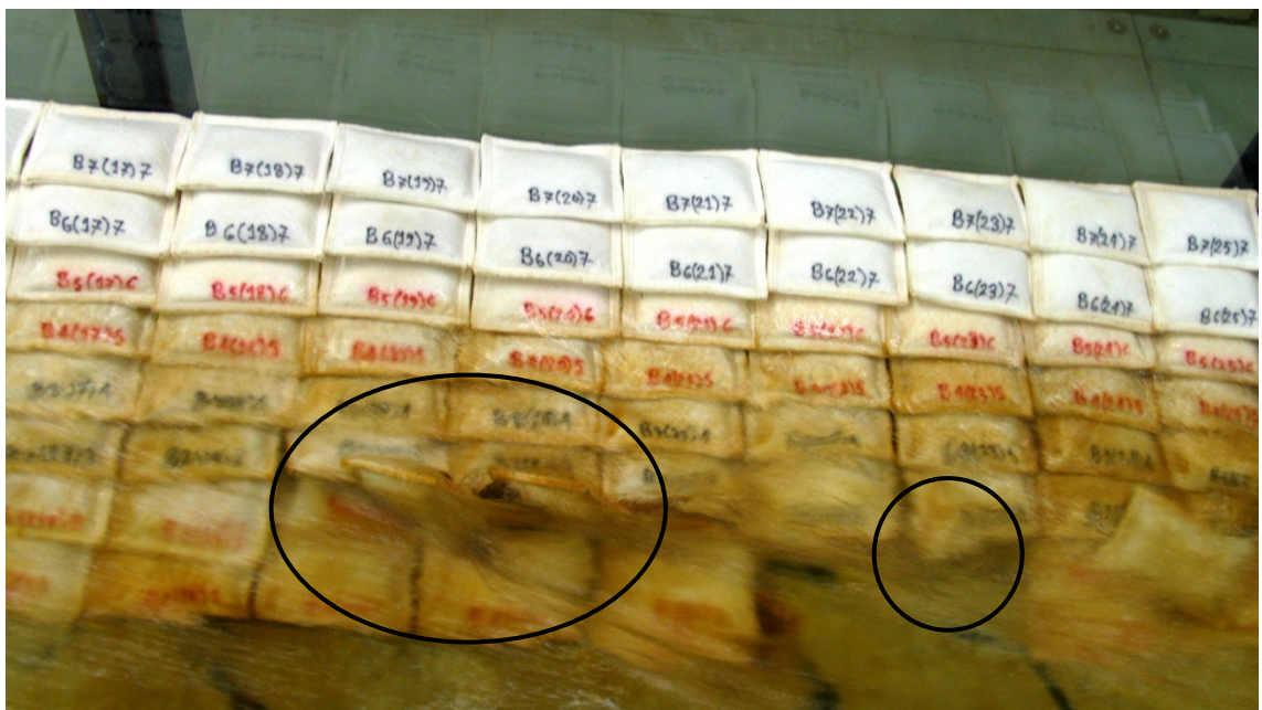
(b) Partial uplifting and sliding
