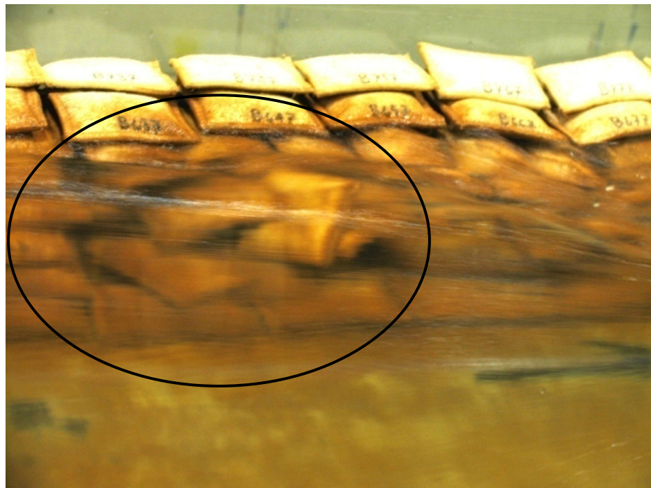
(b) Displacement due to (i) pressure differences between the main and void flow and (ii) sliding
