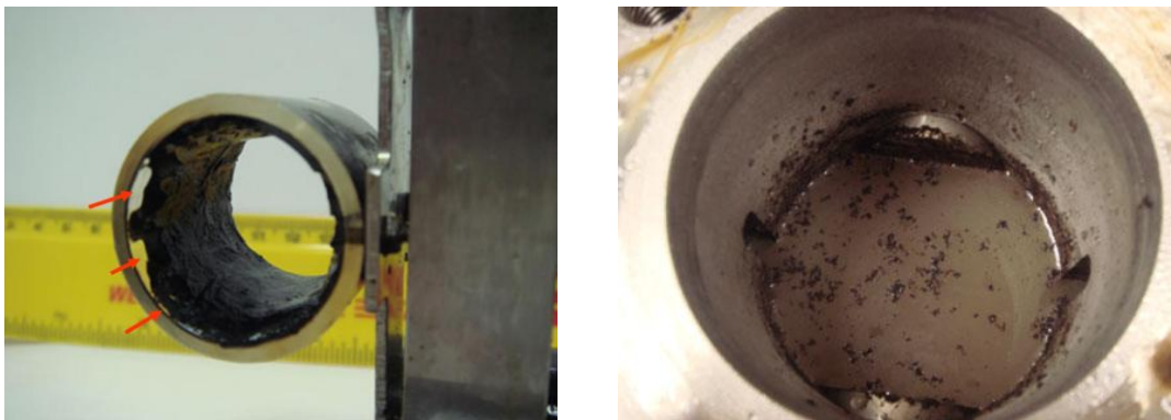
Figure 7.6 Mini tubes impeller and the experimental cell after experiments with varying hydrates concentrations
