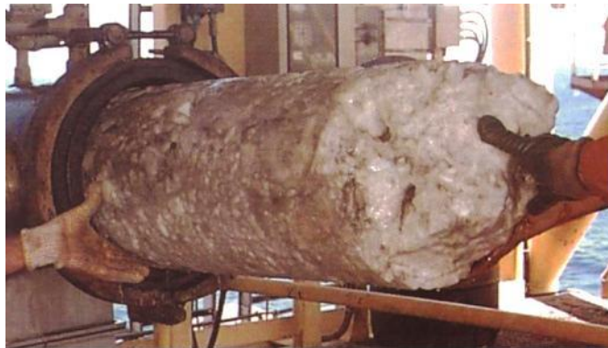
Figure 2.4 Gas hydrate removed from a subsea transfer line (courtesy of Petrobras)
