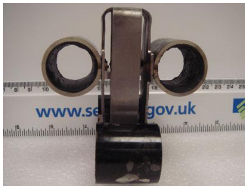
Figure 7.5 Mini tubes impeller and the experimental cell before and after experiments with no hydrate formed.
