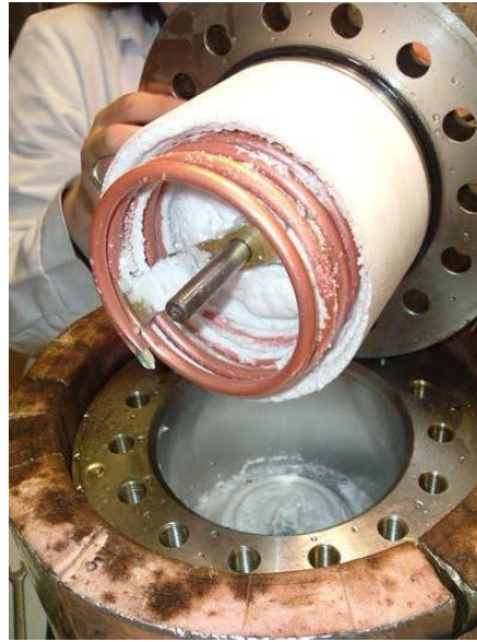
Figure 6.3 An example of hydrate building up on the wall of the HTI setup
