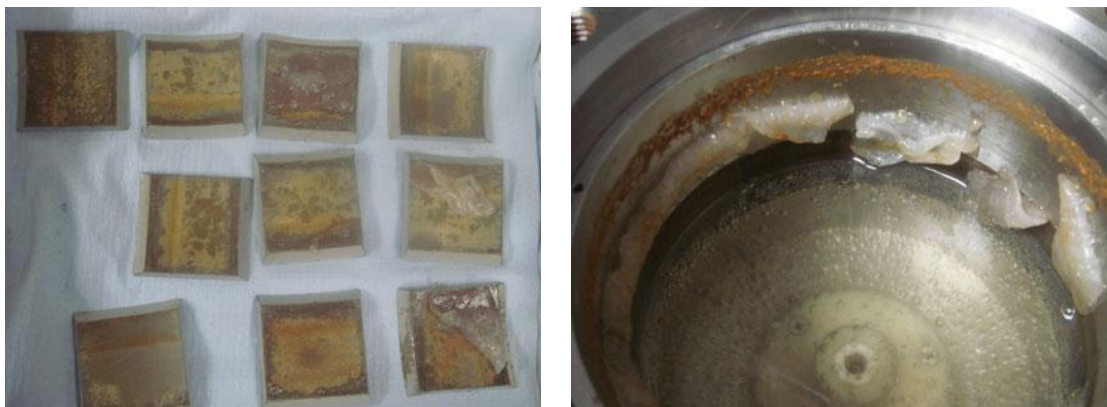
Figure 7.3 Inserts covered with a model wax (grease) before and after experiments
