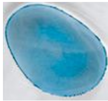
Figure 2.13 Cross-section of Tencel fibre [45]
