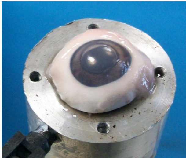
Figure 4-15: Cornea-sclera section suspended over the aluminium cavity
