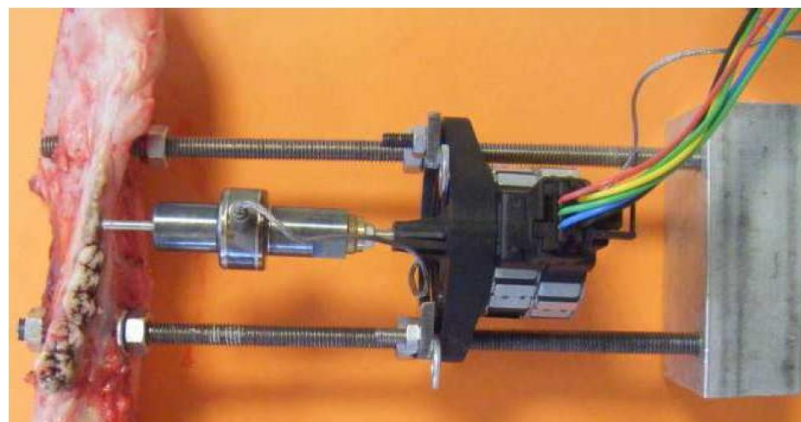
Figure 4-17: Top view of the force relaxation rig with a pig mandible in place [183]
