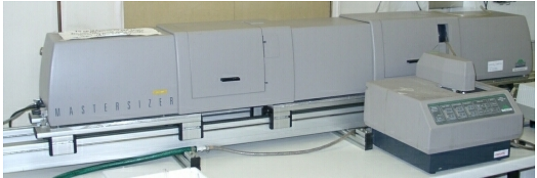
Figure 3.14 Malvern Mastersizer S used for particle size distribution studies
