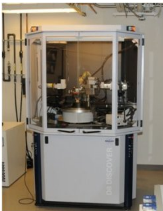
Figure 3.13 Bruker D8 Discover transmission X-ray diffractometer used for XRD analysis
