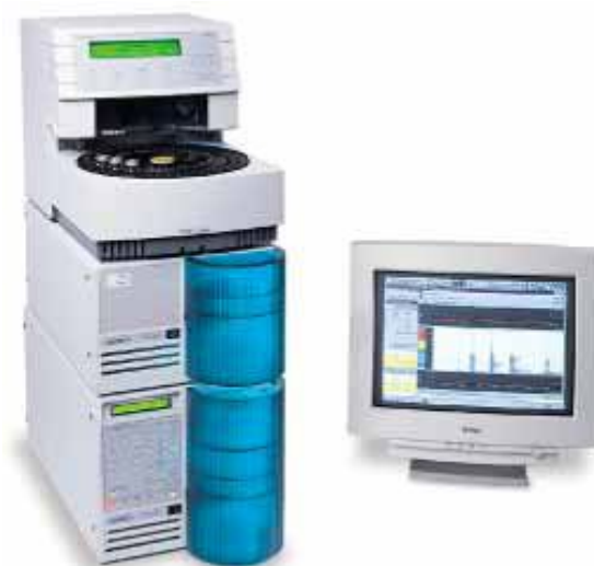
Figure 3.11 Varian Prostar 230 used for HPLC analysis
