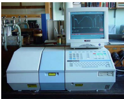
Figure 2.9 The Perkin Elmer Spectrum FT-IR system used (Organic Chemistry laboratory, Heriot-Watt University)
