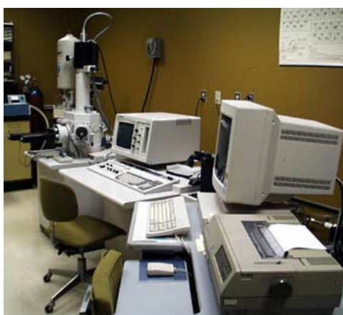
Figure 3.12 Hitachi S-2700 Microscope used for SEM analysis
